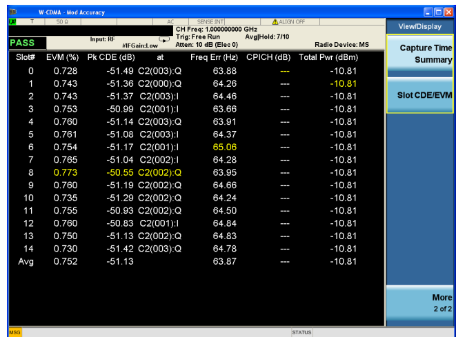
Figure 10. HSUPA capture time summary trace showing error metrics for 15 consecutive slots.
