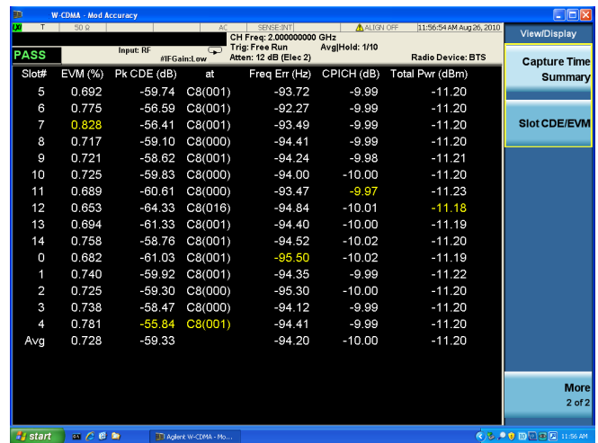
Figure 4. W-CDMA capture time summary trace showing error metrics for 15 consecutive slots.
