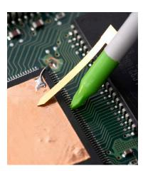
Use a smaller probe tip and a shorter ground connection for reduced noise pickup and inductive loading.
