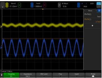
N2873A 10:1 probe on channel 1 (yellow) and N2870A 1:1 probe on channel 3 (blue) measuring 2mVpp 100kHz sine wave.
