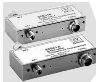
Figure 9. CalPod calibration refresh modules are in-situ devices that can remove the effects of environmental variations in test cables, connectors, adaptors, switch matrices, to re-establish a valid calibration at the measurement plane.
