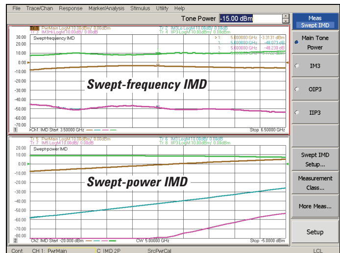
Figure 4. Measures third order IMD and IP3 at 201 frequency (or power) points in a matter of seconds, compared to several minutes using signal generators and a spectrum analyzer.
