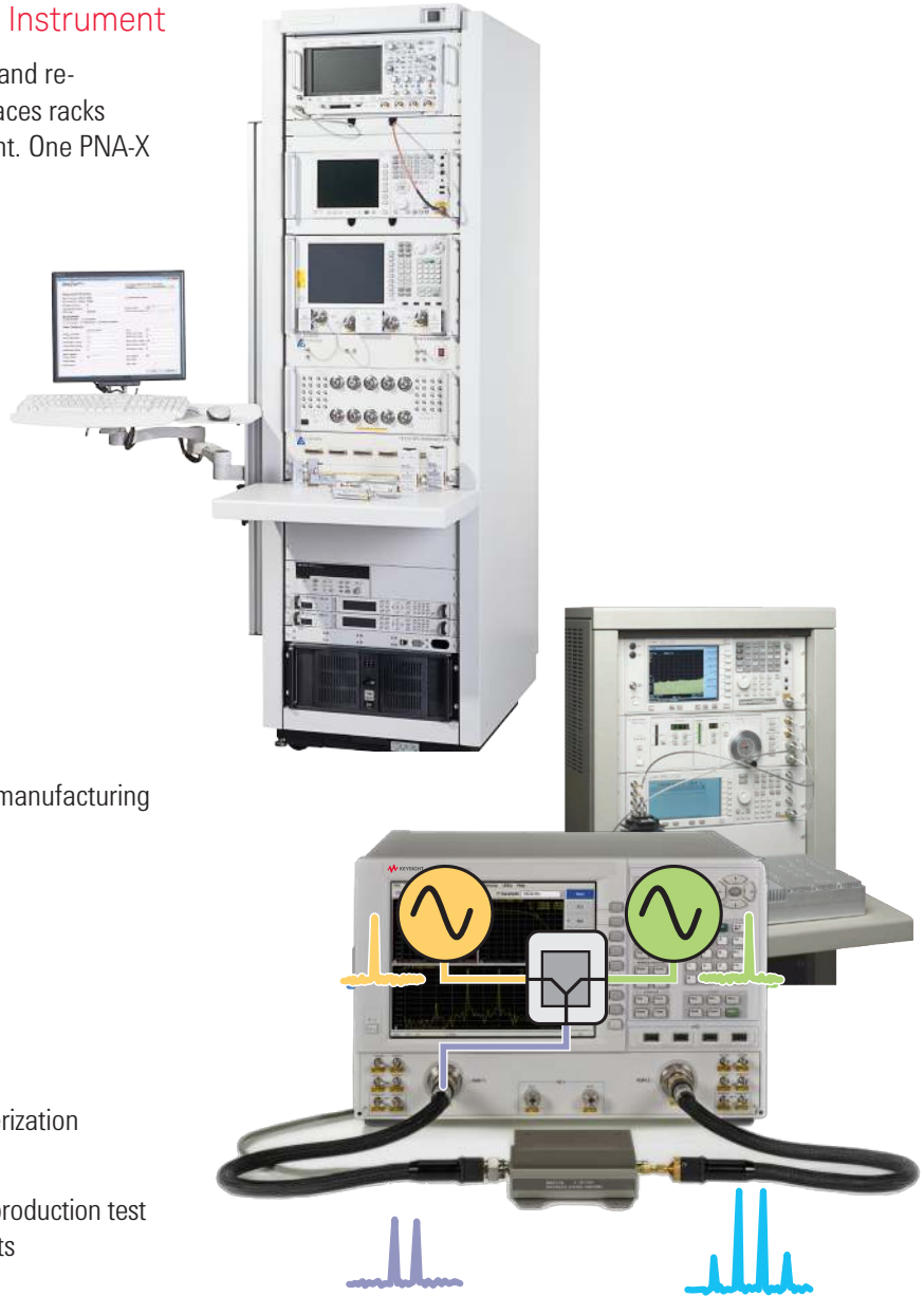
Figure 8. The PNA-X with IMD application replaces two signal generators and a spectrum analyzer in the system rack, simplifying the system configuration and increasing test throughput
