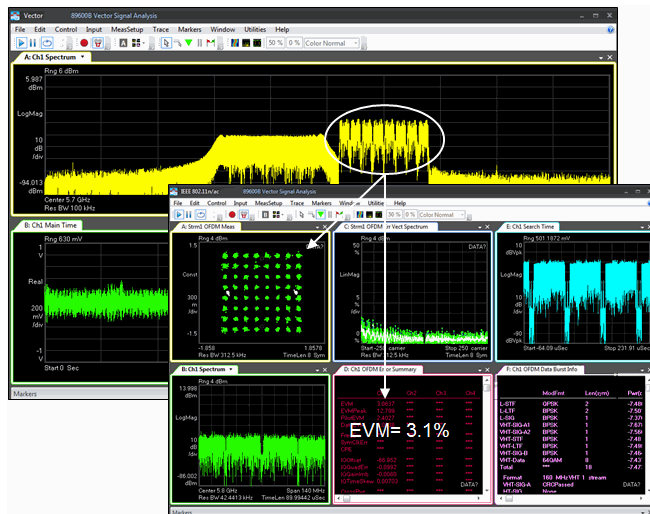
Figure 8. Slight overlap between 802.11ac WLAN and C-band radar signal.
