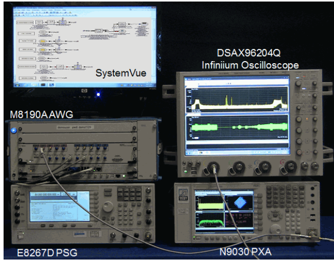
Figure 3. COTS test setup to create and analyzer multi-emitter test signals.
