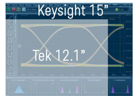
A 15" multi-touch capacitive touch-screen display offers 2x more viewing area and much greater sensitivity to user inputs.
