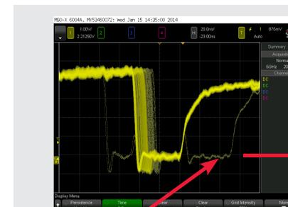
A fast update rate allows you to see an infrequent glitch, but then you want to isolate it. With the 6000 X-Series' hardware zone trigger, you can draw a box to isolate the signal of interest. If you can see it, you can trigger on it.
