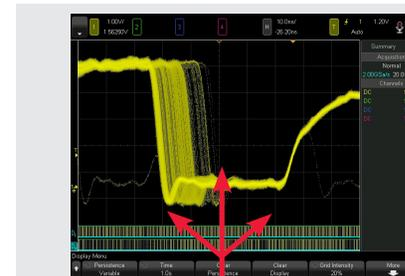
Infrequent glitches and signal jitter captured after one second on 6000 X-Series with standard update rate.
