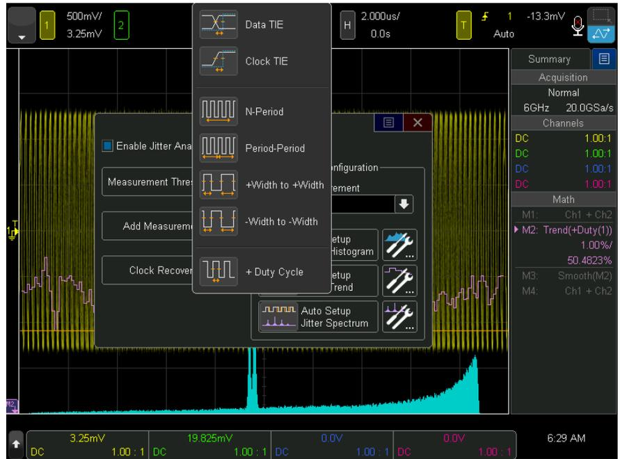
Figure 1. InfiniiVision 6000 X-Series oscilloscope jitter analysis setup menu.
