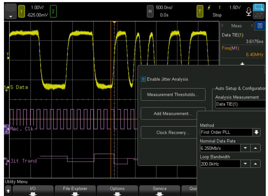
Figure 5. Software-based clock recovery provides a reference waveform for performing TIE jitter measurements.
