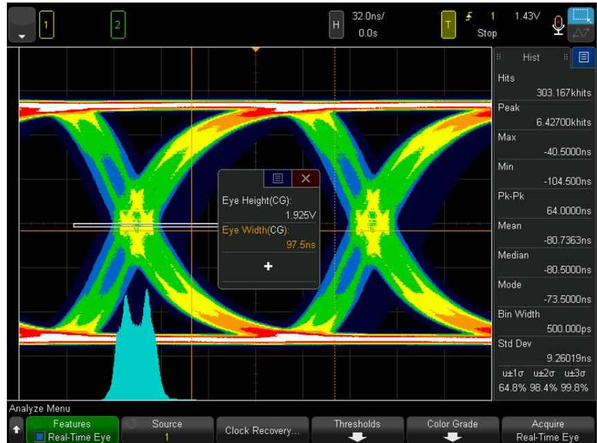
Figure 4. The color-graded real-time eye waveform shows worst-case data valid window (eye-opening).
