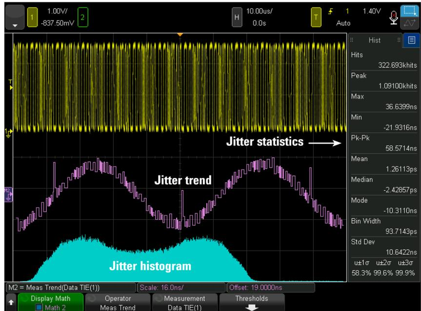
Figure 2. Jitter analysis with the jitter histogram and jitter trend views of timing errors.
