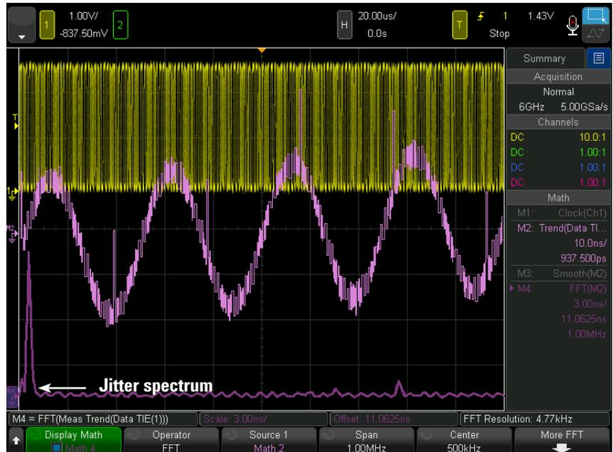
Figure 3. Jitter analysis with the jitter spectrum and jitter trend views of timing errors.
