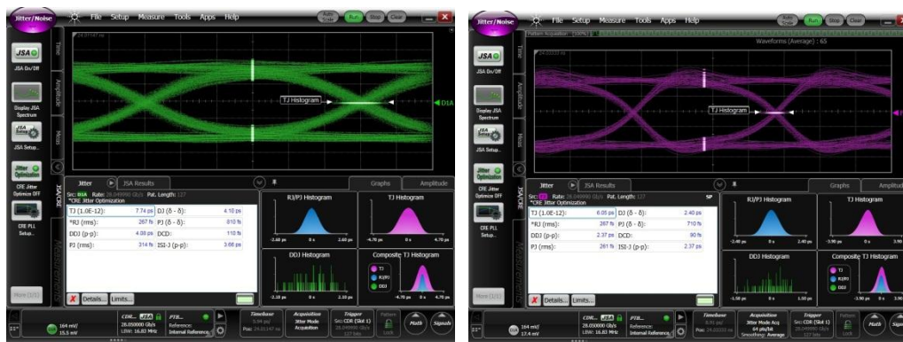
Figure 27: Jitter analysis results on raw signal (left) and de-embedded signal using 1-port AFR model (right).
