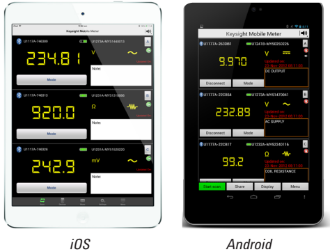
Figure 10. Up to three handheld meters measurements with the Keysight Mobile Meter Application
