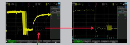
A fast update rate allows you to see an infrequent glitch, but then you want to isolate it. With the 6000 X-Series' hardware zone trigger, you just draw a box to isolate the signal of interest. If you can see it, you can trigger on it.
