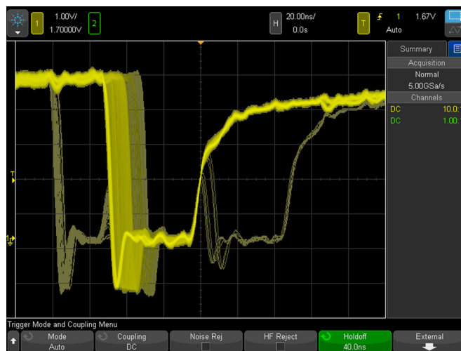
Figure 1: Example of a hard-to-capture signal anomaly with infinite persistence turned on
