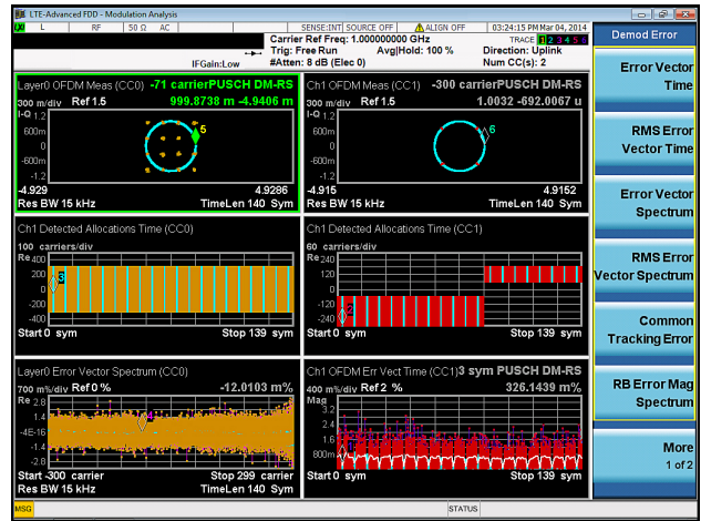
Figure 4. Uplink modulation analysis measurement showing constellation, EVM vs. subcarrier, detected allocation, and EVM vs. symbol information for two component carriers. Measurements are color-coded based on channel type and up to 12 markers with marker coupling between measurements are available for easier troubleshooting.
