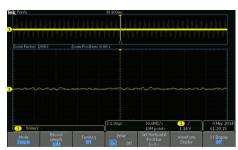
MDO3000's 10 M of memory can't maintain sufficient sample rate to accurately capture the 250 bursts over 1 second.
