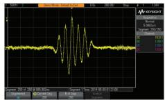
3000 X-Series captures 250 bursts and almost 1 second of time at 5 GSa/s with segmented smart memory, which allows the 3000 X-Series to easily reproduce the waveform without undersampling.
