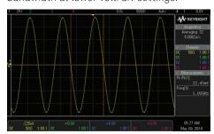
3000 X-Series measures 22.4 mV p-p on a 1 GHz sine wave at 3 mV/div.
