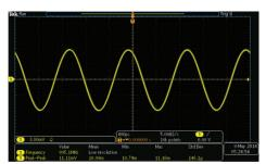
MDO3000 measures 11.1 mV p-p on the identical 1 GHz sine wave at 3 mV/div due to severe bandwidth limiting.
