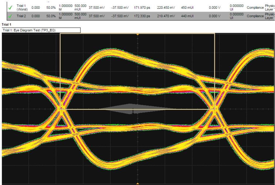
Figure 12. Summary report detail: The eDP 1.4 software's summary report provides screen shots of all the measurements that have been performed. In this figure, you can see the data-eye. Observe the clear status and description at the top and the measurement data just above the eye.
