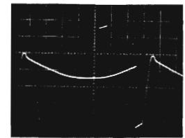
F. Same as C, except Q7 fires later due to smaller load (2v, 3a)
