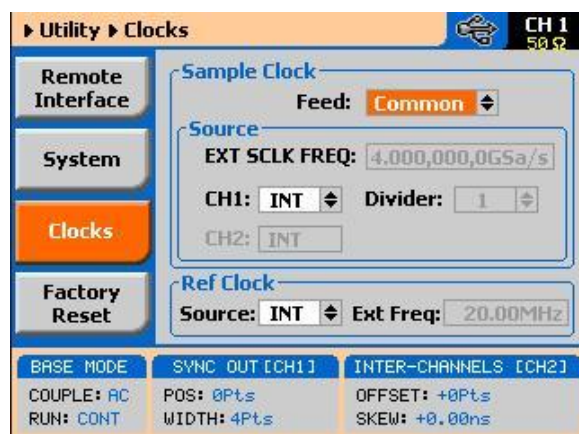
Figure 3-16: Modifying the SCLK and 10MHz Clock Source
