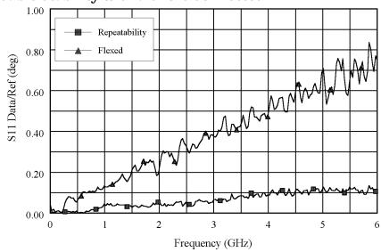
Figure 9-3 Cable Stability with a Short Connected
