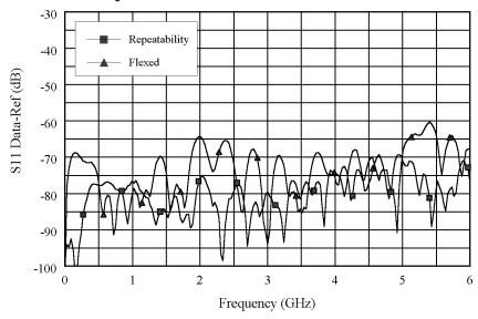
Figure 9-1 demonstrates the concepts useful in determining cable reflection stability. A fixed load is connected to the free end. The DATA-MEM feature provides an indication of the cable reflection stability. A 60-dB peak on the chart yields a reflection stability estimated as  $10^{(-60/20)}$  or 0.001.
