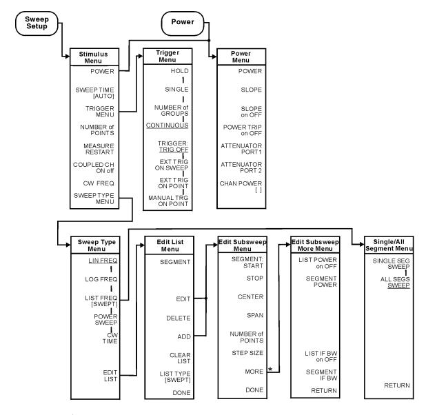
Figure 3-8 Menu Map for Power and Sweep Setup
