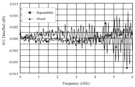
Figure 9-2 Cable Stability with a Short Connected
