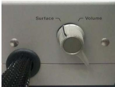
Figure 4. Selector switch of the N1424 Volume/Surface selector box.
