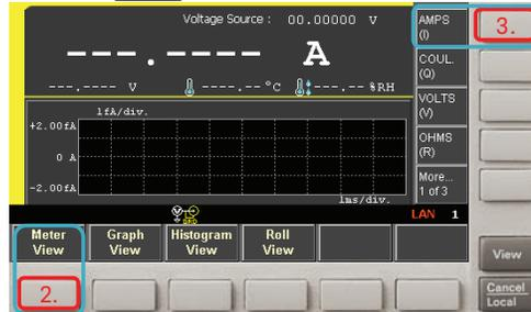
4. (1) Check if the Voltage Source field is set to 0 V.
