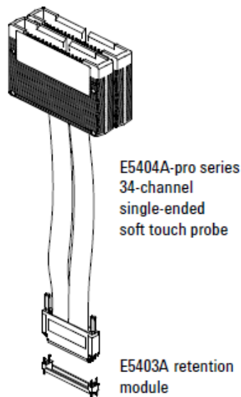
Figure 3 E5404A-pro series single-ended soft touch probe and E5403A retention module
