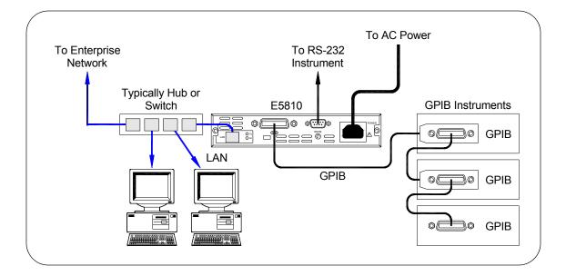
After connecting the E5810 to the Enterprise network, plug the E5810 AC power cord into an AC outlet and observe the power-on sequence. When the power-on sequence is complete, the assigned IP address of the E5810 is displayed on the second line of the front panel display. A typical display follows. See Chapter 1, "E5810A Description" for power-on sequences.
