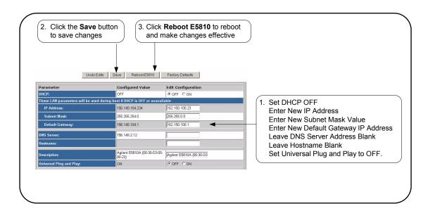
Configuring the E5810 for Local Network Operation If you plan to install your E5810 on a Local network, use the **Configuring** your E5810 LAN/GPIB Gateway page to set the parameters applicable to your Local network.
