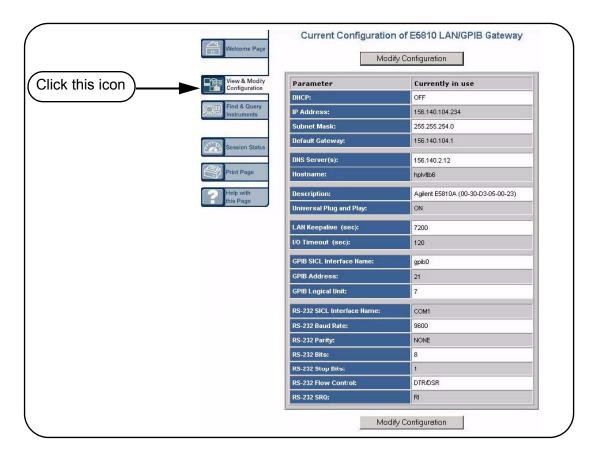
3 Display the Modify Configuration Page. From the Current Configuration of E5810 LAN/GPIB Gateway page, click the Modify Configuration button to display the Password dialog box.
