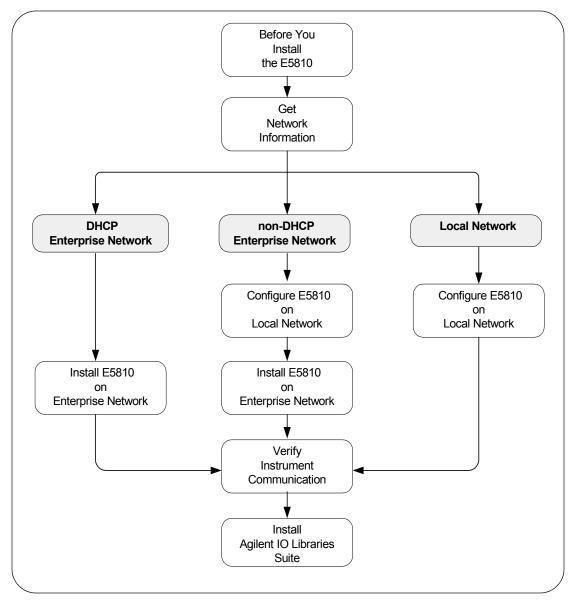
You can install the E5810 on an Enterprise (corporate) network that supports Dynamic Host Configuration Protocol (DHCP), an Enterprise network that does not support DHCP, or a Local network.
