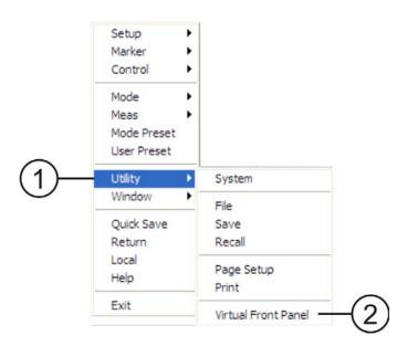
On the VFP the keys labeled "Key 1" through "Key 7" function as the menu keys. Using the mouse to click on a combination of the VFP keys and the menu keys on the display screen, you can operate the instrument as if it had conventional front-panel keys.
