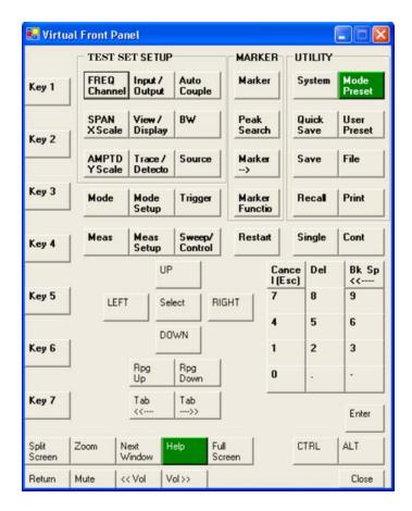
When you click a button in the Virtual Front Panel, it performs the operation of the corresponding test set front-panel key. The buttons at the left of the panel, named Key 1 through Key 7, perform the operation of the respective softkeys. The Rpg Up and Rpg Down keys perform the operation of the knob.
