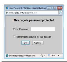
By default, this password is set at the factory as "agilent". However, you may subsequently change the password. (Press **System**, **I/O Config**, **Reset Web Password** on the test set front panel to change the password.)
