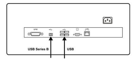
In addition, the Agilent IO Libraries CD that was included with your test set contains USB Host drivers that allow control of other test sets connected to the USB bus.
