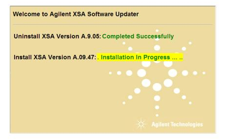
The new instrument software is being installed. The "Installation in Progress" text will roll across the screen indicating software activity. There will be several windows appearing and disappearing during this time. NO interaction with the instrument is required. Please be patient the total software installation process can take 30 to 40 minutes. It will display "Completed Successfully" when the software update is complete. You will be prompted to restart you instrument at the end.
