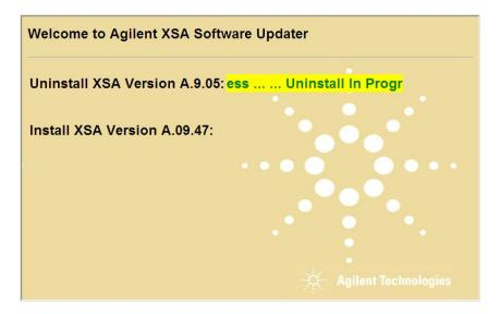
The old instrument software is being uninstalled. The "Uninstall in Progress" text will roll across the screen indicating software activity. There will be several windows appearing and disappearing. It will display "Completed Successfully" when this step is finished.
