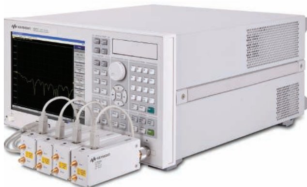
Using four U1810B's to extend a 4-port ENA to 8 ports to increase throughput
