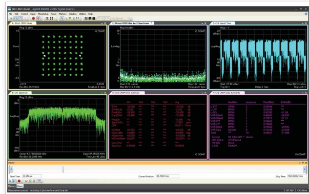
Figure 11. This segment of the recorded spectrum contained minimal noise and the demodulated 802.11ac signal was in good condition.
