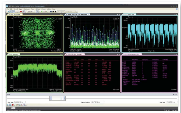
Figure 13. This portion of the recorded spectrum shows the presence and effects of a broadband interference signal.
