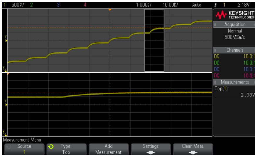
Figure 46 Isolating area for Top measurement
