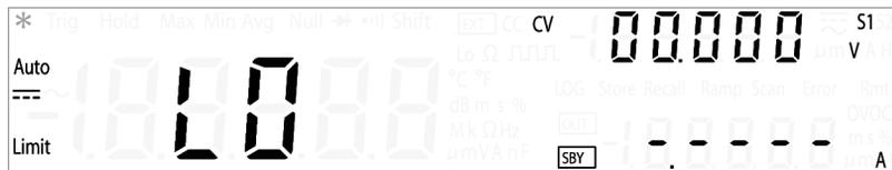
Each time the input value transitions from “PASS” to “HI” or from “PASS” to “LO”, or when transitioning directly from “HI” to “LO” or “LO” to “HI”, the instrument beeps once (if the beeper is enabled).
