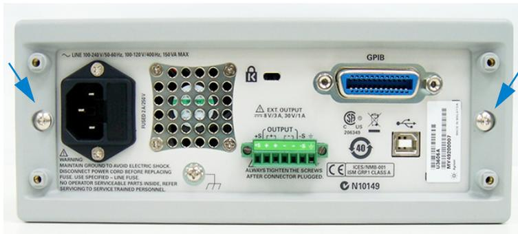
**5 Remove the cover.** Remove the screws in the bottom of the cover.
