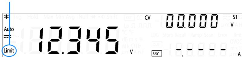
The primary display briefly shows “PASS” when readings are within the specified limits, “HI” when the reading is above the high limit, and “LO” when the reading is below the low limit.
