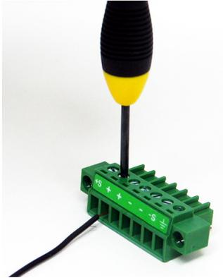
*Do not use the shield as one of the sensing conductors. Ground the shield at the U3606A end only. The other end of the shield should be left unconnected. Observe the polarity when connecting the sensing leads to the load. You can connect the output leads to either one of the two + or - terminals. They are internally shorted.*
