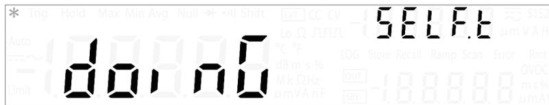
If the self-test fails, the Error annunciator illuminates.
