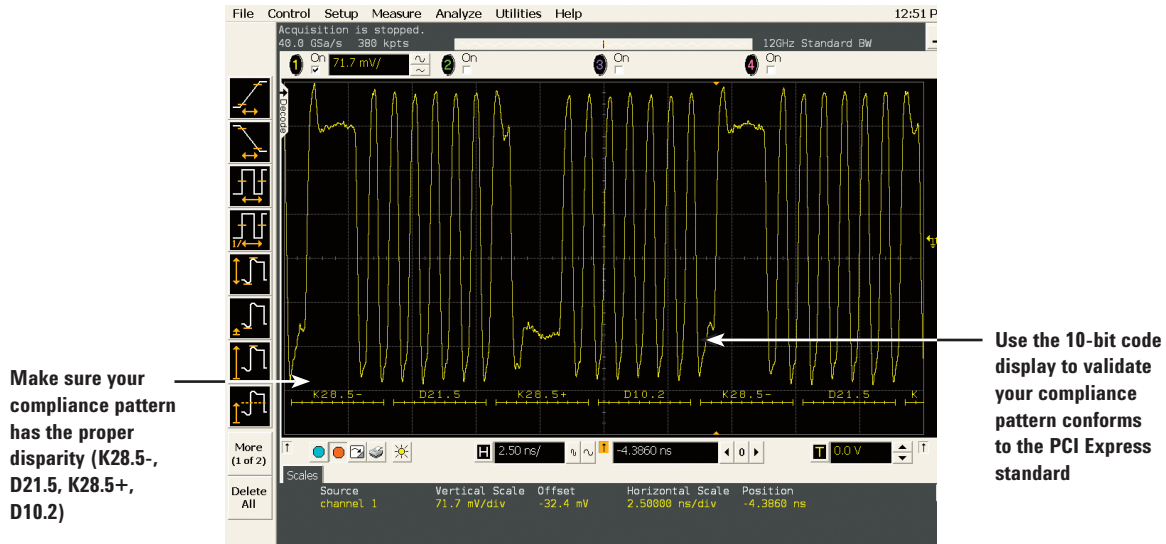
Figure 24. The 8b/10b decoded symbol information is shown below the appropriate portion of a PCI Express signal using the E2688A software.
