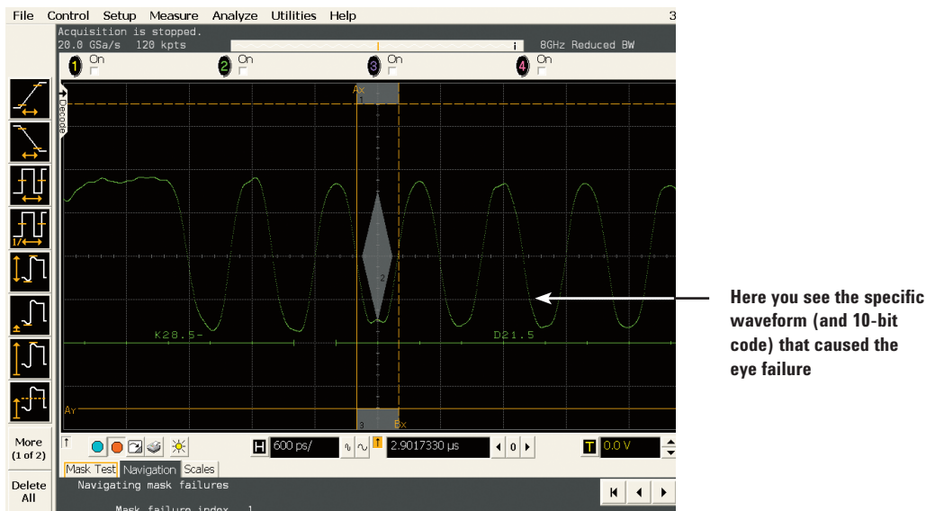
Figure 27. The E2688A allows you to show the specific waveform that caused an eye diagram failure.
