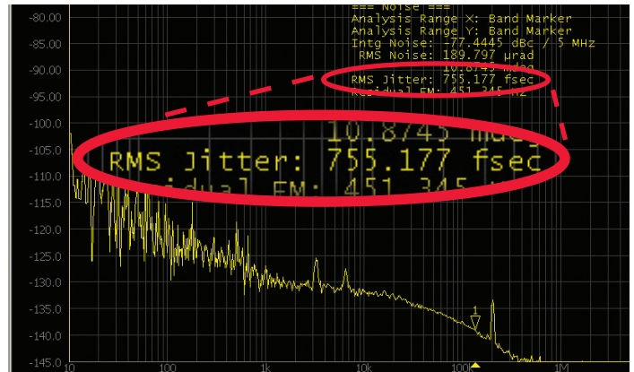
Figure 2. Signal source analyzer measurement screen.
