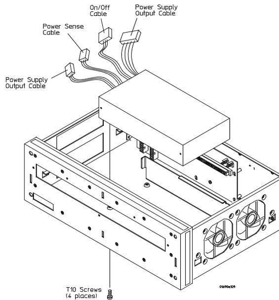
**6** Reverse this procedure to install the power supply
