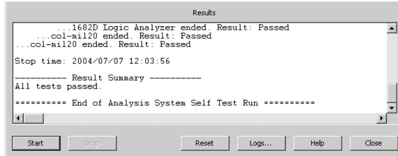
The self tests can be run one at a time by clicking on the self-test of interest. The results of the individual test will be reported under Results. For example, if you select the Serial Memory Test and the highest reporting level, the following results should be reported in the status window:
