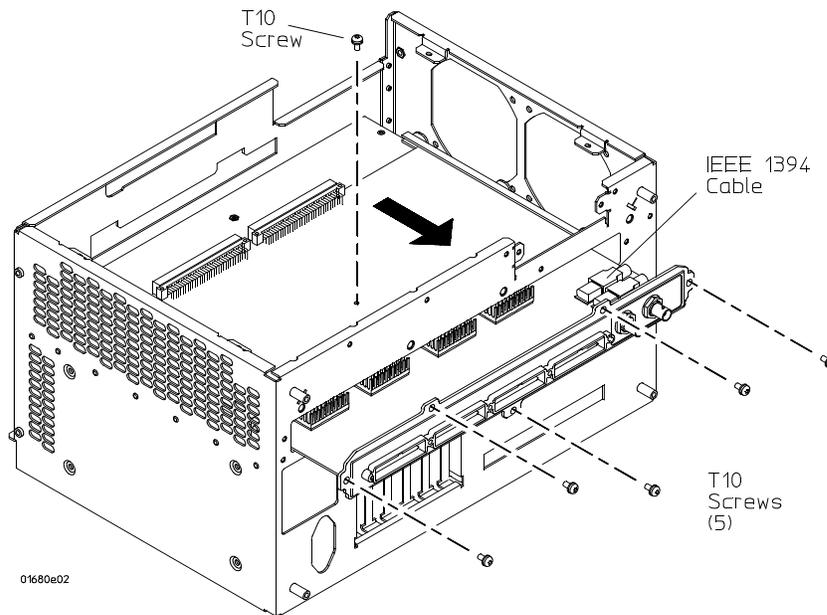
Steps to remove probe shroud from acquisition board.
