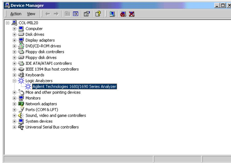
If the logic analyzer device is not listed, then uninstall and reinstall the Agilent Logic Analyzer application software. If the device still does not appear, then there is a problem with the Windows XP Professional operating system. Consult the documentation for the operating system to determine why the device is not being installed and run.
