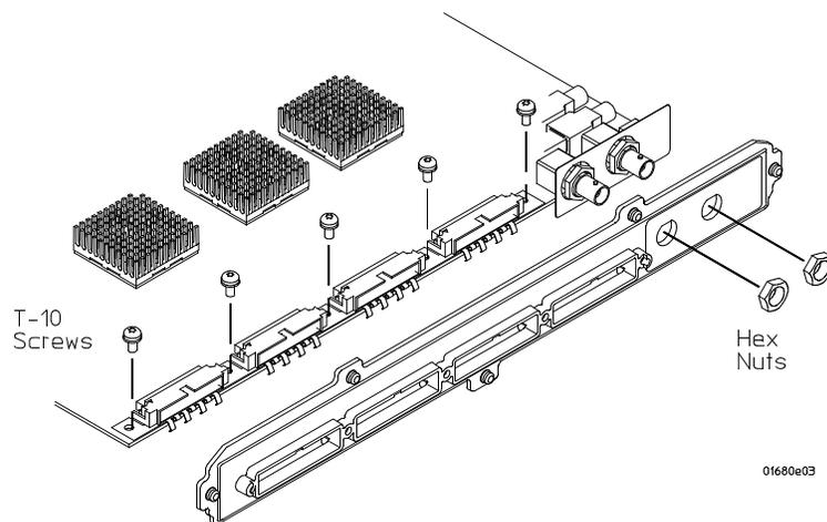
Reverse this procedure to install the acquisition board.
