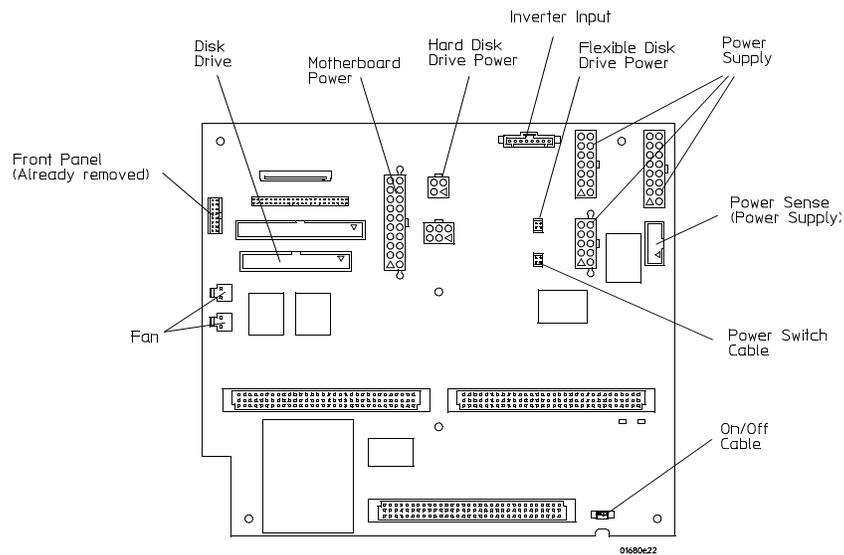
**3** Using a Torx T-10 screwdriver, remove six screws that secure the distribution board to the chassis.
