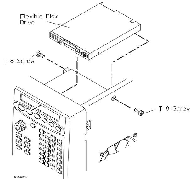
When installing a new flexible disk drive, industrial double-sided tape (Agilent 0460-2010 or similar) is required to dress the cable onto the flexible disk drive. Apply the tape as shown.
