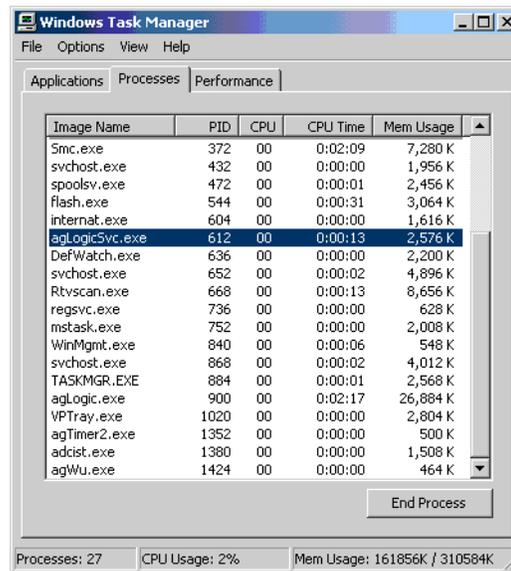
If the agLogicSvc service is not listed, then uninstall and reinstall the Agilent Logic Analyzer application software. If the agLogicSvc service still does not appear, then there is a problem with your Windows XP Professional operating system. Consult the documentation for the operating system to further determine why the service is not being installed and run.
