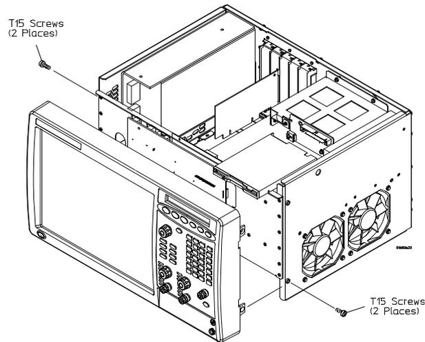
**6** Reverse this procedure to install the front panel assembly.
