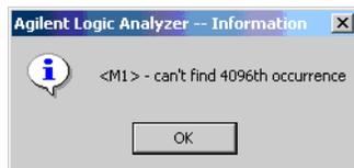
When the above error message appears, one or more samples of test data is incorrect. When this happens, check the following and attempt the test again:
