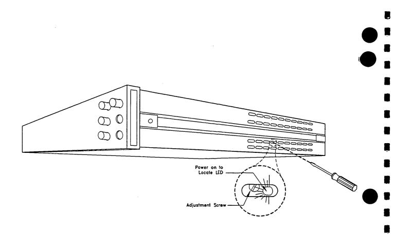
Figure 4-1. 10x Voltage Output Adjustment Location
