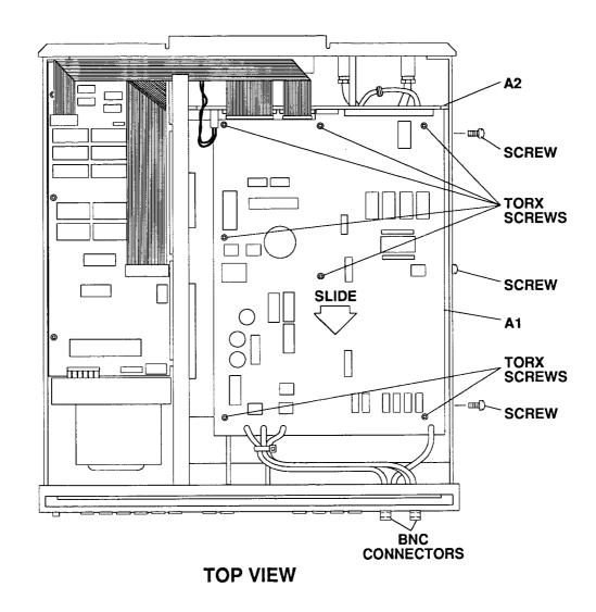
Figure 3-4. Remove and Replace A1/A11 Inguard Source PCA
