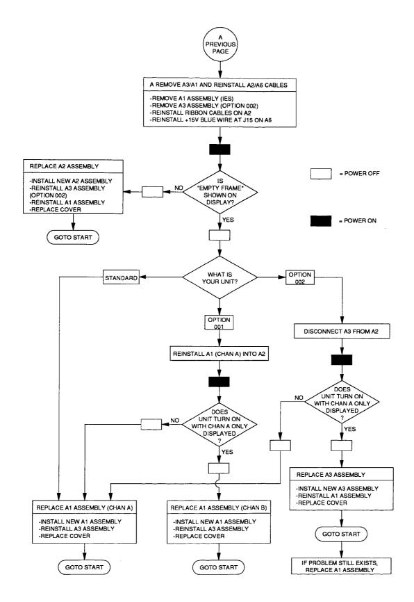
Figure 3-2. Turn-on Failure Troubleshooting Diagram (2 of 2)
