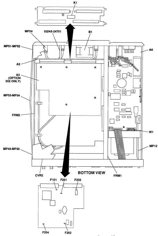
Figure 2-3. Universal Source Parts, Bottom View
