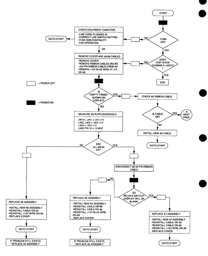
Figure 3-2. Turn-on Failure Troubleshooting Diagram (1 of 2)
