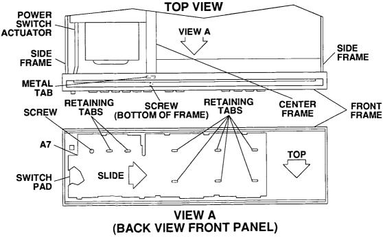
Figure 3-9. Remove and Replace A7 Display Logic PCA
