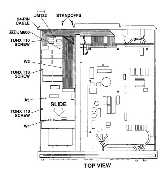
Figure 3-7. Remove and Replace A5 Outguard Logic PCA
