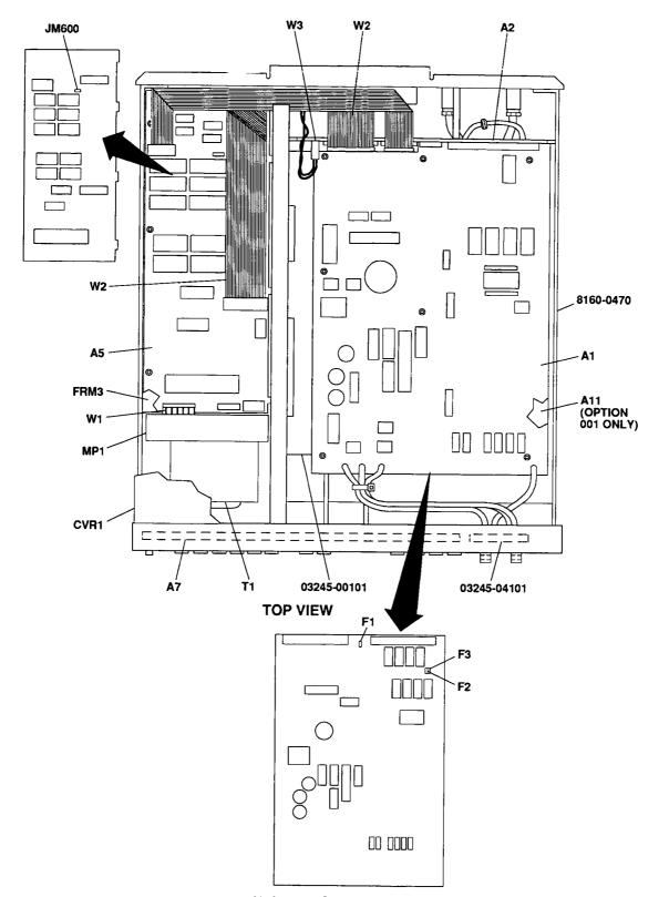
Figure 2-2. Universal Source Parts, Top View
