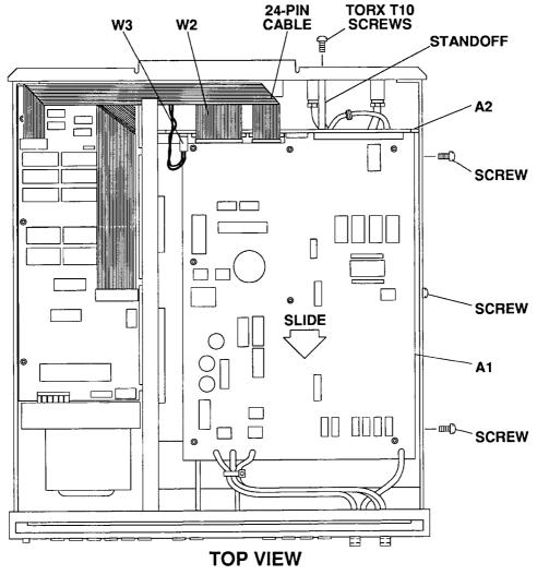
Figure 3-5. Remove and Replace A2 Backplane PCA
