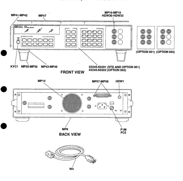
Figure 2-1. Universal Source Parts, Front/Rear View
