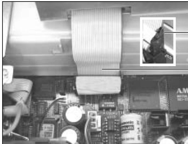
Snap the Locking Clips over the top of the connector to secure the Ribbon Cable
