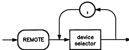
where the device selector is the address of the instrument appended to the HP-IB port number. Typically, the HP-IB port number is 7, and the default address for the synthesizer is 19, so the device selector is 719.
