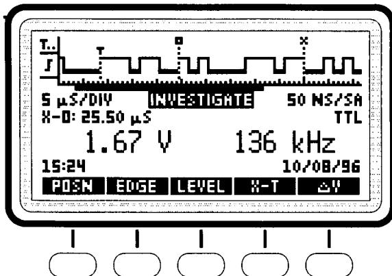
Press the menu key below the label to perform that action. In the display above, pressing the right hand menu key, labeled **ΔV**, turns on or off the ΔV measurement (described on page 10).
