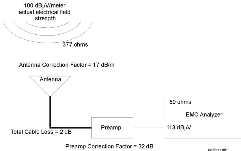
In order to transfer the measured signal amplitude to the true signal level it is necessary to correct for the following:
