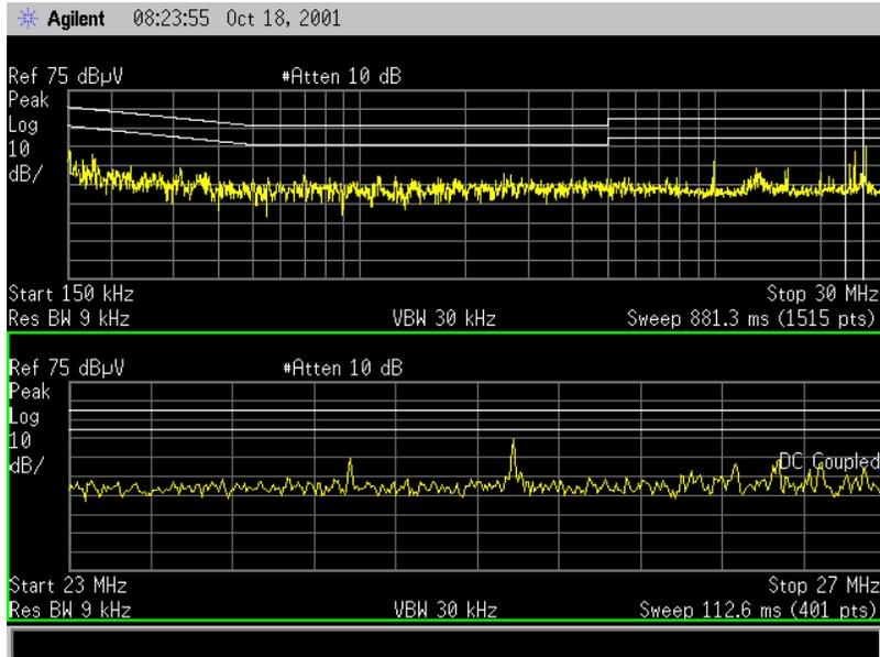
8 Measure the Peak, Quasi-peak, and Average level of signals near or above the limit.
