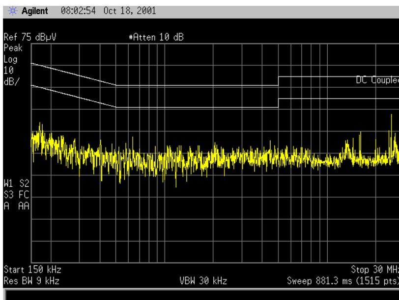
If no EUT signals appear above the lower (Average) limit line on the EMC analyzer display and you have verified that the EMC analyzer is not in IF or RF overload (see next section), then the product passes the conducted emissions limit.
