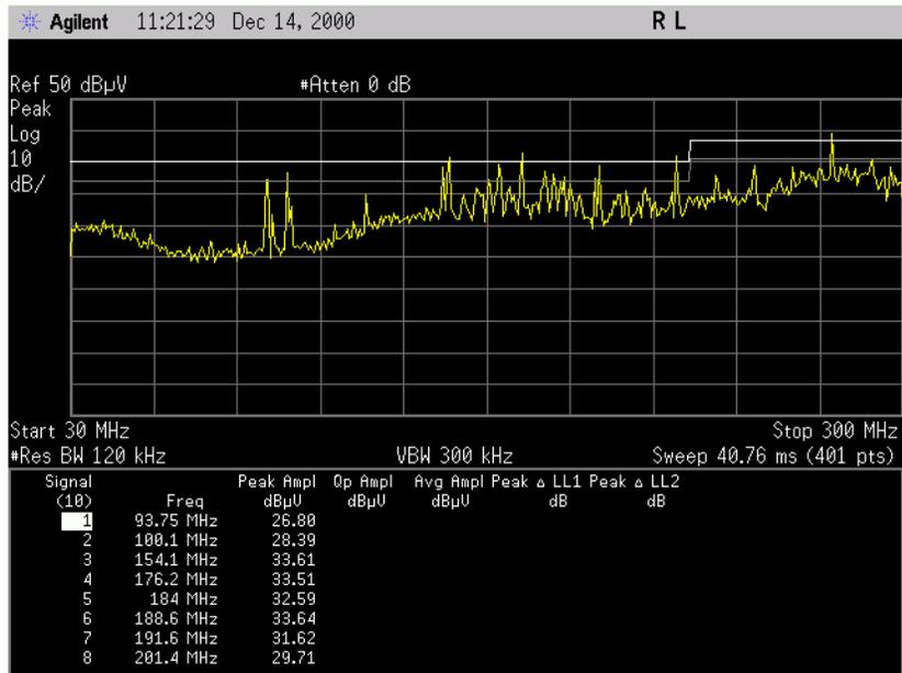
When the automeasure process is complete, the emissions above the limit line margin will be displayed in the signal list with the measured peak amplitude.
