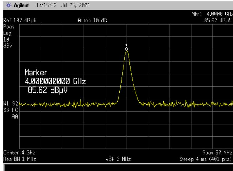
In Figure 4-5 the analyzer reads a value of 85.62 dB $\mu$ V which is within the stated specifications ( $\pm 0.54$  dB absolute amplitude accuracy +  $\pm 1.5$  dB absolute frequency response).
