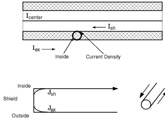
At low frequencies the current is evenly distributed throughout the conductor. But at higher frequencies, the skin effect enables the cable shield to provide additional protection. Here, most of the return current flows on the inside of the shield because it is the surface closest to the center conductor in which the signal current flows.
