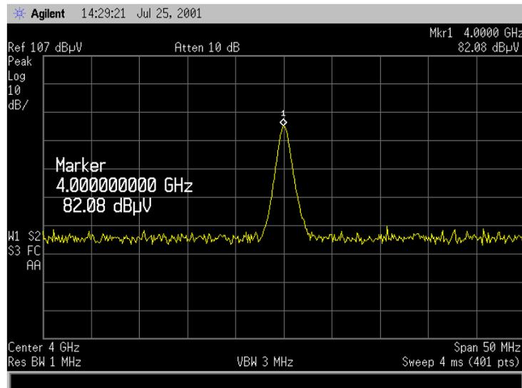
In Figure 4-4, the analyzer reads a value of 82.08 dB $\mu$ V which is below the actual input signal level. In this case, the Preselector filter has not been centered for best amplitude accuracy.
