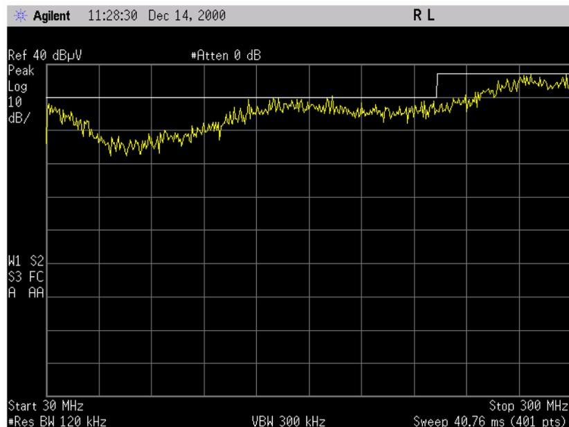
6. If you have adequate limit line to noise floor separation without using preamplification, and do not wish to use a preamp, you may skip the rest of these steps. If the noise floor to limit line separation is not adequate for measuring your emissions, you may need to add internal or external preamplification.
