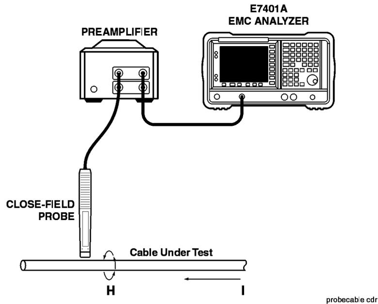
Use the close field magnetic probe to determine the magnetic field intensity around a cable. The current density can then be calculated if the distance from the center of the cable to the center of the probe loops is known.
