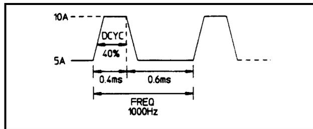
Figure 5-5. Continuous Transient Operation
