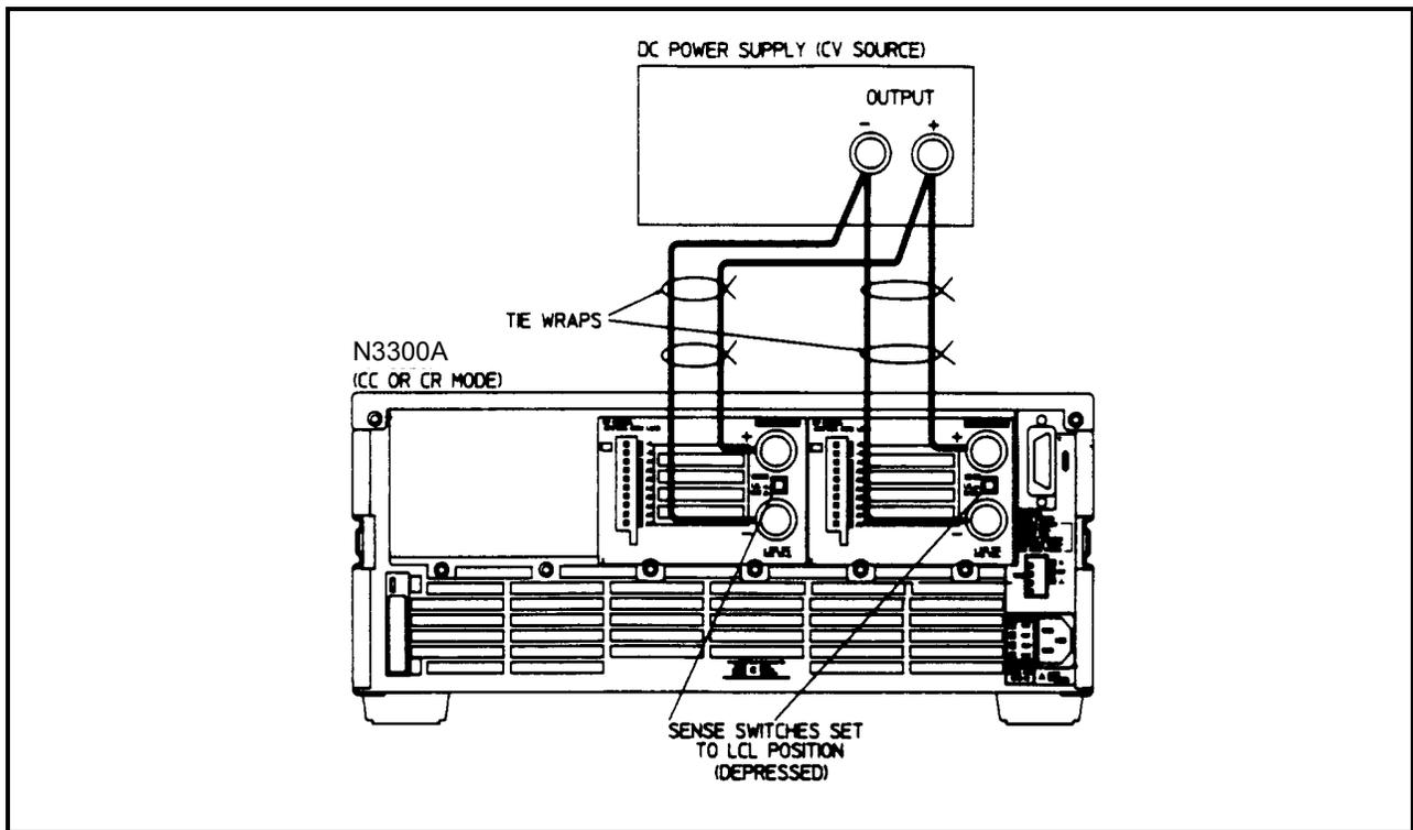
Figure 3-12. Parallel Operation
