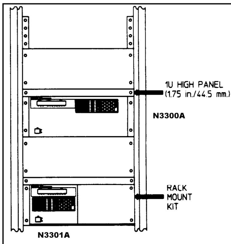
Figure 3-4. Rack Installation
