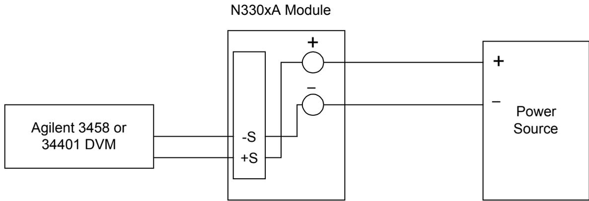
Be sure sense switch is in RMT position
