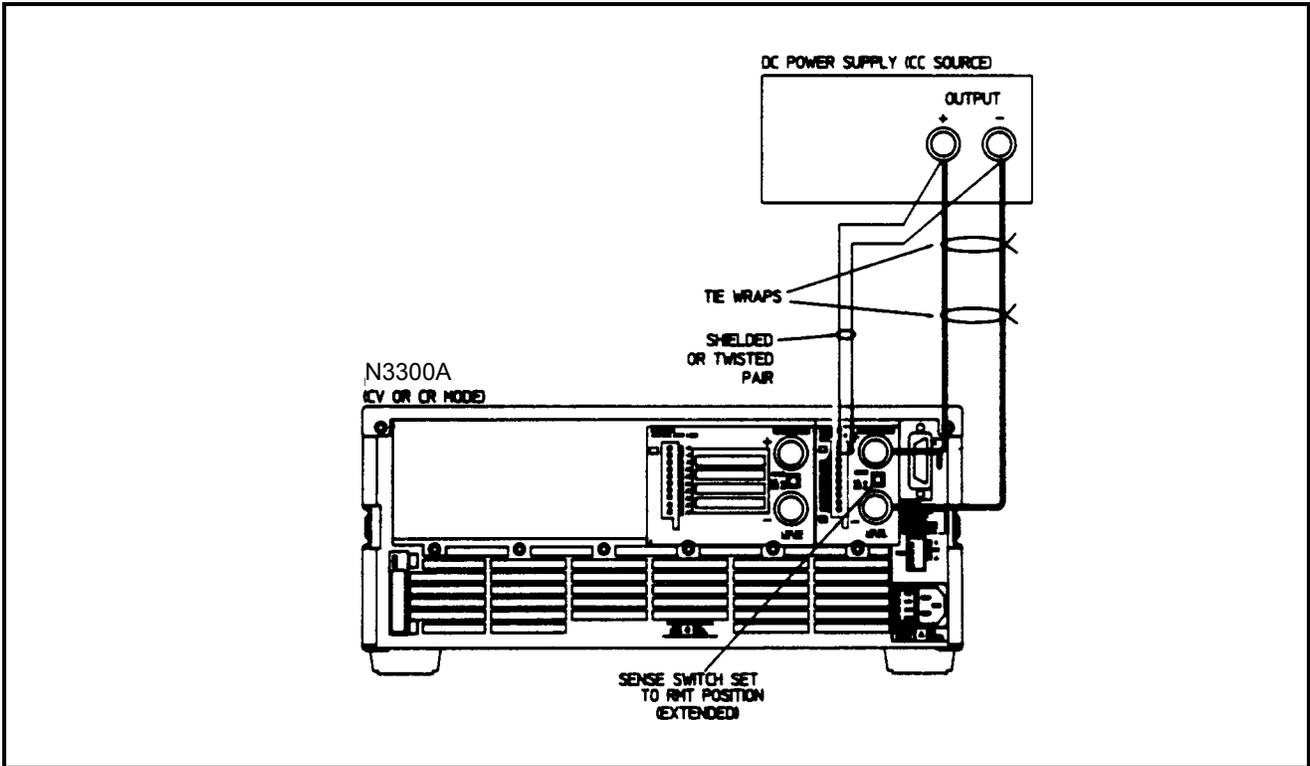
Figure 3-11. Remote Sensing
