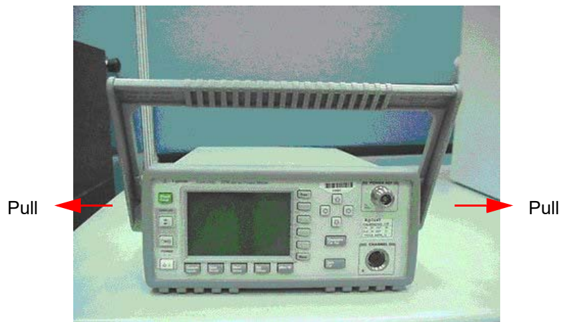
Figure A-2 Remove the power meter handle
