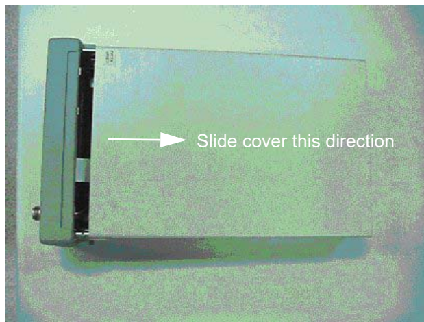
Figure A-3 Remove the power meter cover
