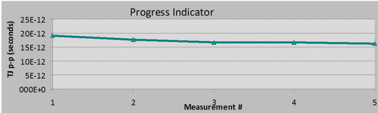
Figure 7 – Progress Chart indicating good stabilization of total jitter results.
