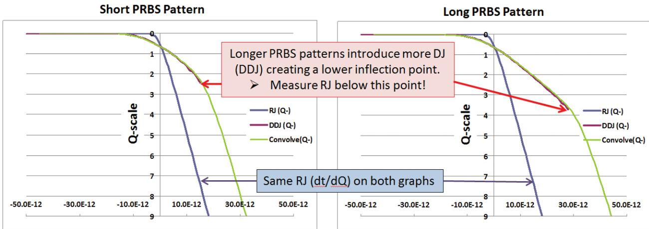
Figure 5 – Increasing PRBS pattern length increases DDJ and lowers the inflection point on a Q-scale plot.
