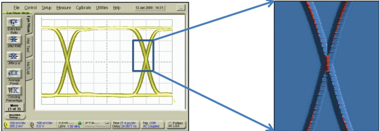
Figure 1 – The 3D Color Grade Scale (CGS) database in Eye/Mask mode creates a PDF of the incoming signal.
