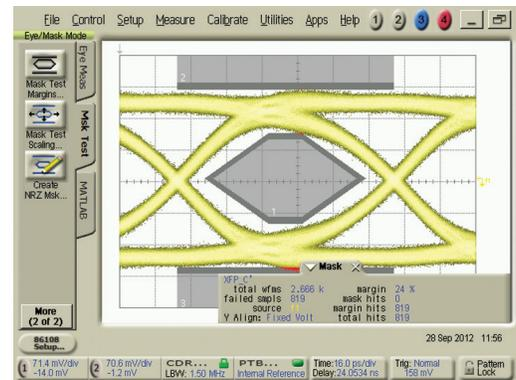
Figure 6b - Right: Traditional eye mask testing expands a mask to determine mask margin.
