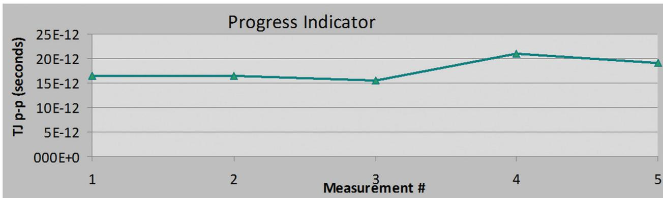
Figure 8 – Progress Chart indicating additional measurement time (more samples) is required to yield an accurate result.
