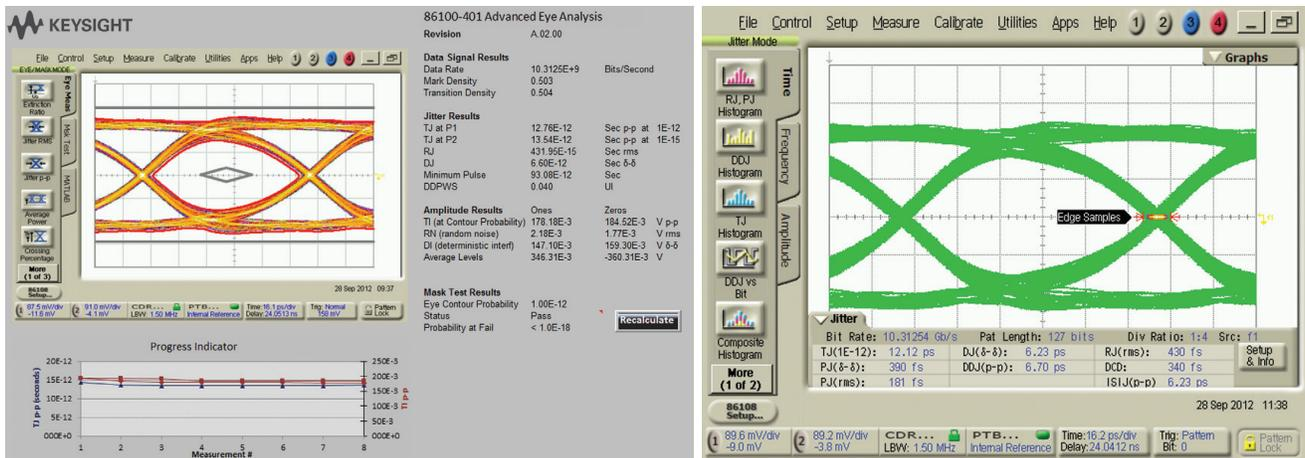
Figure 14 - Measurement performed using a PRBS7 pattern for both RJ and DJ measurements (Steps 1 and 2). TJ @ 1E-12 = 12.76 ps p-p (Option 401) / 12.12 ps p-p (Option 200 only).
