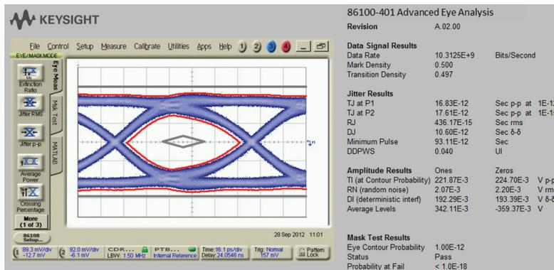
Figure 6a Eye diagram showing BER contour lines (red lines) and BER-based mask (grey lines).
