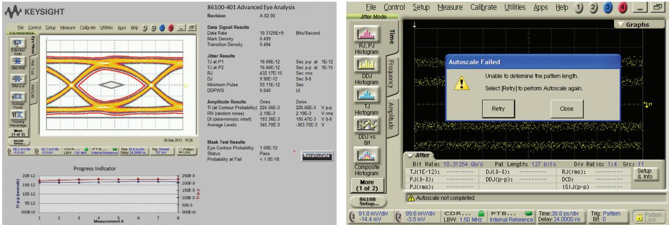
Figure 16 - Jitter results using a PRBS-31 pattern (PRBS7 pattern used for RJ measurement in Step 1). TJ @ 1E-12 = 16.06 ps p-p (Option 401) / Exceeds pattern length limitation (Option 200).
