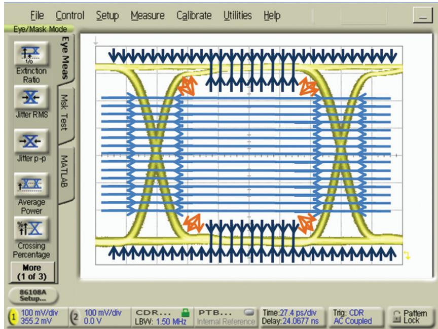
Figure 3 – Eye diagram showing CGS data that contains jitter information only (horizontal arrows), amplitude information only (vertical arrows), and samples heavily influenced by both jitter and amplitude effects (diagonal arrows).
