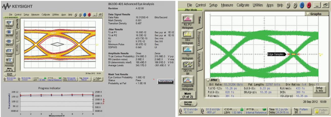
Figure 15 - Jitter results using a PRBS-15 pattern (PRBS7 pattern used for RJ measurement in Step 1). TJ @ 1E-12 = 15.55 ps p-p (Option 401) / 15.26 ps p-p (Option 200).
