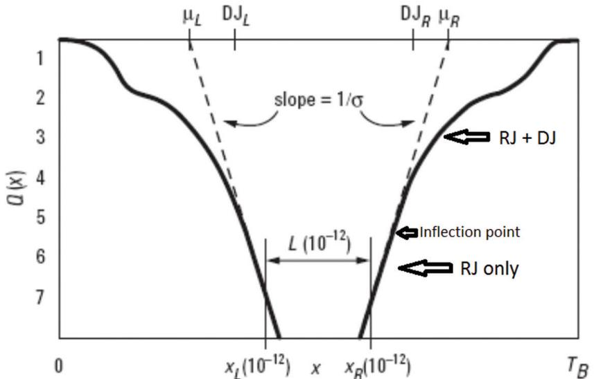
Figure 4 – When plotted on a Q-scale, the data will be a straight line when it is dominated by random jitter effects.
