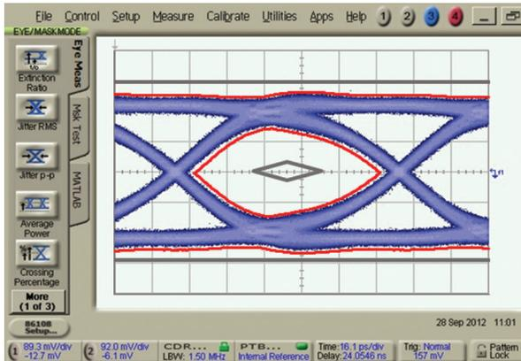
Today's devices are characterized using a variety of test patterns. A commonly used test sequence for jitter and eye analysis is the Pseudo-Random Binary Sequence (PRBS) having  $2^{31}-1$  bits in length. Why test using PRBS-31? PRBS patterns are easy and inexpensive for devices to generate using hardware, and a long pattern like PRBS-31 ( $2^{31}-1$  bits, or 2,147,483,647 bits) includes bit sequences that effectively stress baseline wander and clock wander in devices.
