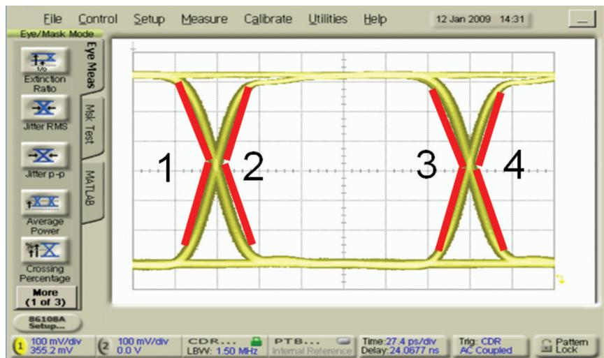
Figure 2 – Eye diagram showing edges containing jitter information.
