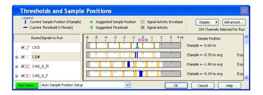
Setting the signals CA9\_0\_R and CA9\_0\_F automatically adjusts all of the other Command and Address buses/signals. (There is no need to adjust STAT, ROWADDR, COLADDR, COMMAND, COMMANDO, BA, AB, AP or any other command or address bus signal.)
