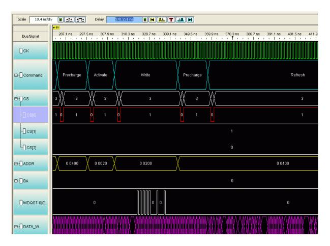
4 To check that all of the Write Data bits are aligned, configure the target to generate write-only traffic with an alternating 0/1 bit pattern. If necessary, select a different eye opening so that each DQ signal is sampled at the same time. In the following example, the first data bit needs to be adjusted:
