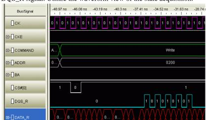
4 Once the read data sample positions are selected, find the correct sample for the DQS\_R signal. Utilize the waveform view of the state acquisition.
