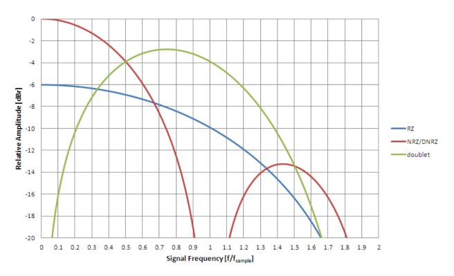
Figure 1-5: DNRZ/NRZ/RZ/Doublet Frequency Response
