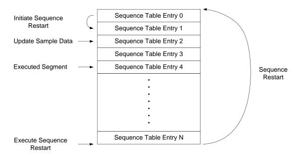
Figure 5-3: Sequence used as Ring Buffer
