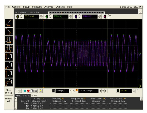
Figure 4-9: Start and stop of frequency sweep
