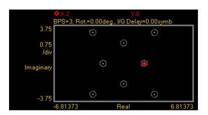
The following example illustrates another possible use of custom modulation to define a distorted constellation. In this particular case, a  $0-\Omega PSK$  modulation with a quadrature error (non-perpendicular I and  $\Omega$  axis) is defined:
