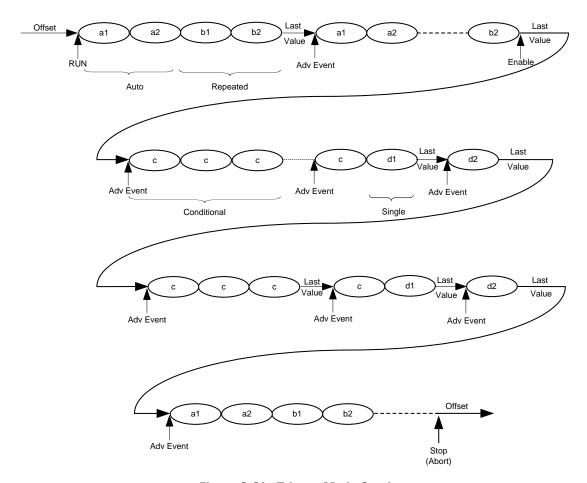
Figure 3-31: Trigger Mode Continuous
