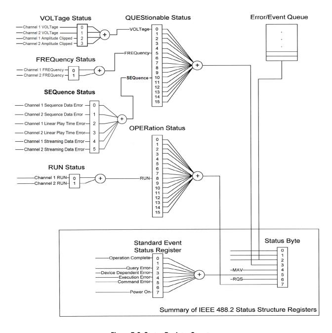
Figure 7-2: Status Register Structure
