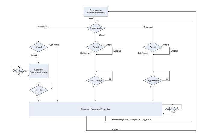
Figure 3-8: Sequencer execution flow
