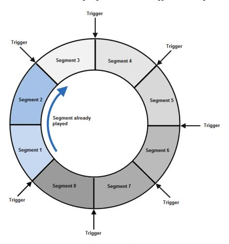
Figure 5-2: Triggered Streaming
