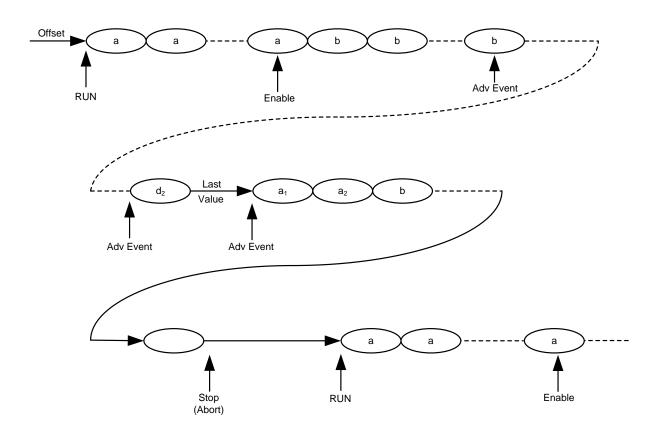
Figure 3-26: Trigger Mode Continuous
