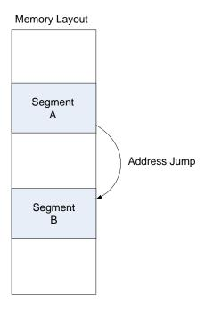
Figure 3-34: Address jump within segments
