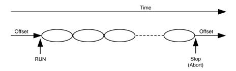
Figure 3-10: Trigger Mode Continuous
