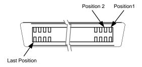
Figure 3-4: DYNAMIC CONTROL IN connector
