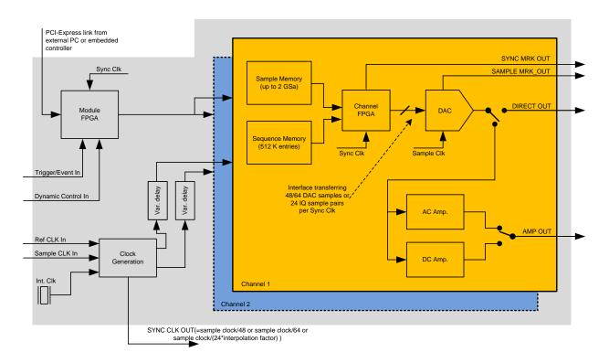
Figure 1-3: M8190A Block Diagram
