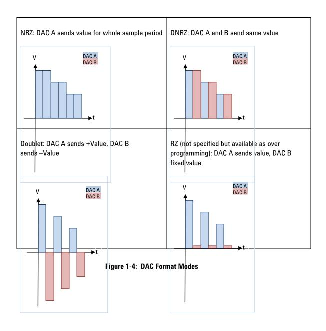
The four modes have different amplitude vs. frequency responses, which are shown in the figure below.
