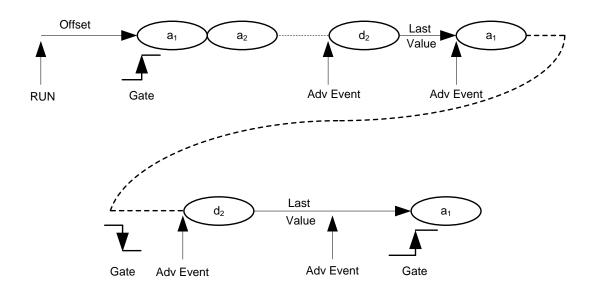
Figure 3-25: Trigger Mode Gated
