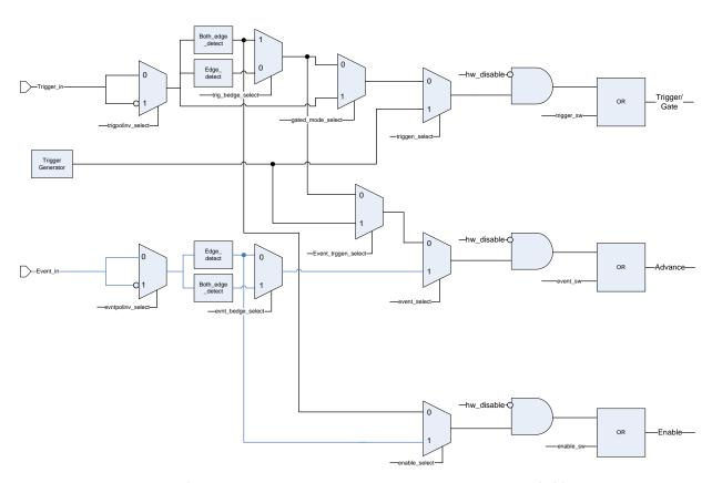
Figure 3-7: Logical input connectivity options provided by M8190A
