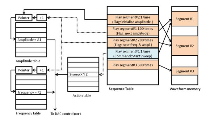
Figure 4-2: Mechanisms to Change Configuration at Run-Time
