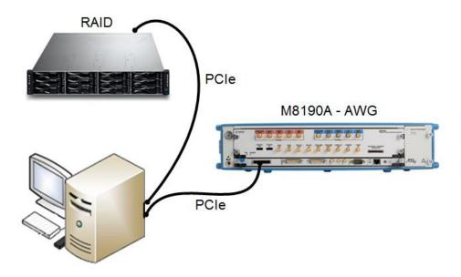
Figure 5-4: Sample Data Storage Using a Raid System
