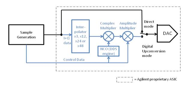
Figure 4-1: Hardware Structure of Features for Digital Up-Conversion
