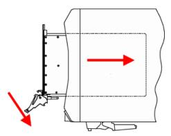
Figure 2-3 Installing the module to the chassis
