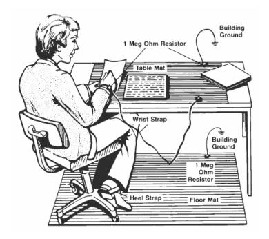
Figure 2-1 Static-safe work station example
