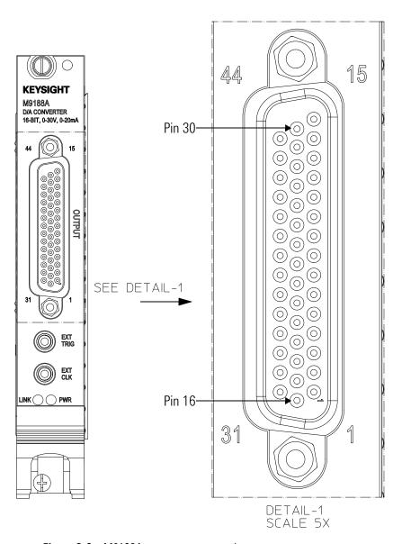
Figure 2-6 M9188A output connector pinout
