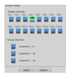
**5** To stop the DC voltage output from Channel 4, toggle the Output Relay, Single Channel: CH4 button to **0FF**. This will turn off the signal and disconnect the output relay.
