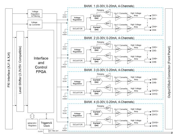
Figure 2-7 M9188A functional block diagram
