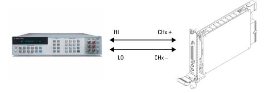
Figure 3-1 Connections For M9188A verification
