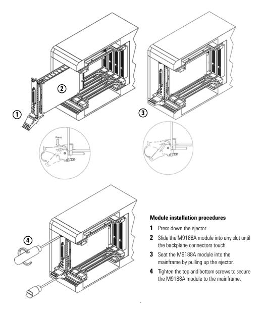
Figure 2-4 Module installation procedures
