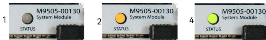
If the chassis does not power up to a steady green Status light, or powers up to a steady red light as shown below, the chassis has a failure and requires service.
