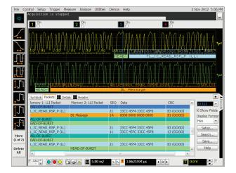
Quickly move between physical and MIPI LLI protocol layer information using the time-correlated tracing marker. Display protocol content using embedded decode in the waveform area, or see protocol events in a compact listing format. Minor tick marks indicate clock transitions. Major tick marks indicate segments of the serial packet MIPI LLI measurements are automatically time-correlated with measurement on other scope channels.
