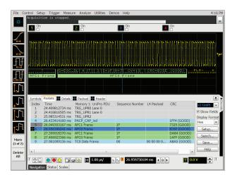
Quickly move between physical and MIPI UniPro protocol layer information using the time-correlated tracing marker. Display protocol content using embedded decode in the waveform area, or see protocol events in a compact listing format. Minor tick marks indicate clock transitions. Major tick marks indicate segments of the serial packet. MIPI UniPro measurements are automatically time-correlated with measurement on other scope channels.
