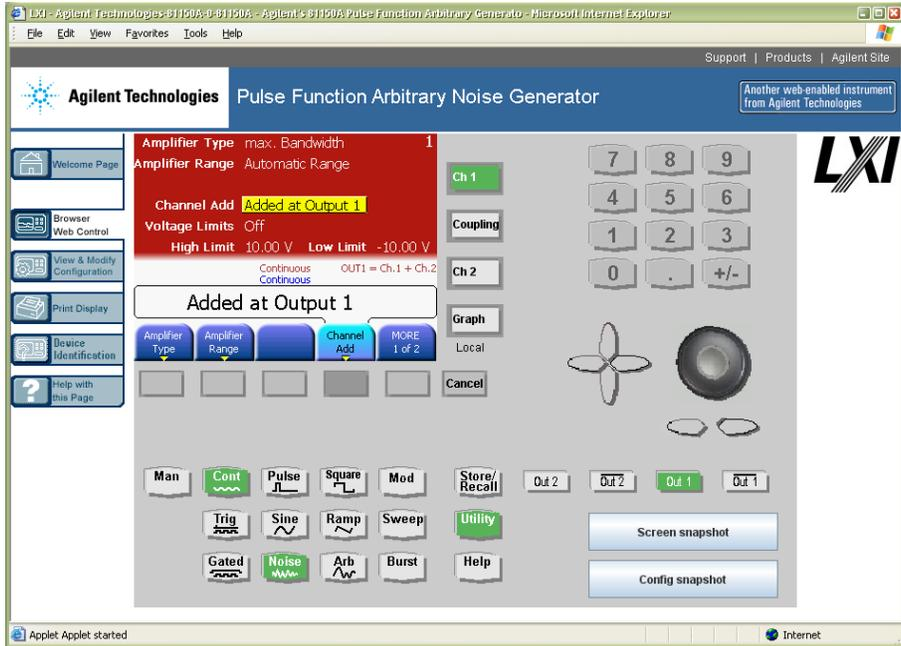
Figure K-3: Agilent 81150A remote interface with channel add feature turned on.
