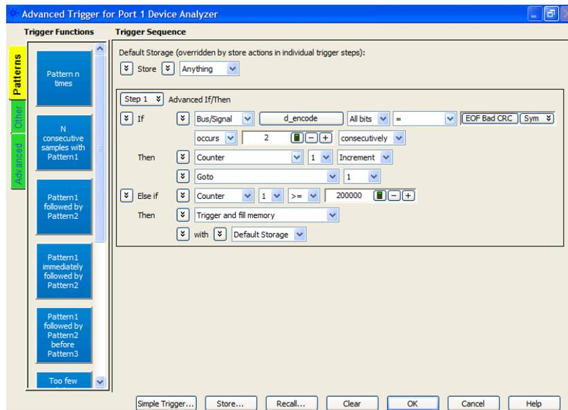
The underlying idea of this trigger definition is to use one of the logic analyzer's internal real-time counters to count frames with wrong checksum (EOF Bad CRC). Based on the N4219B design this event will occur twice for each frame. To count the number of events correctly it is important to know that EOF Bad CRC will occur 2 times in a consecutive manner for 1 wrong frame.
