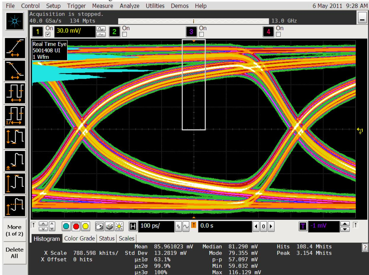
Figure B-4: Gen1 Histogram Example for Upper Inner Eye (not calibrated)
