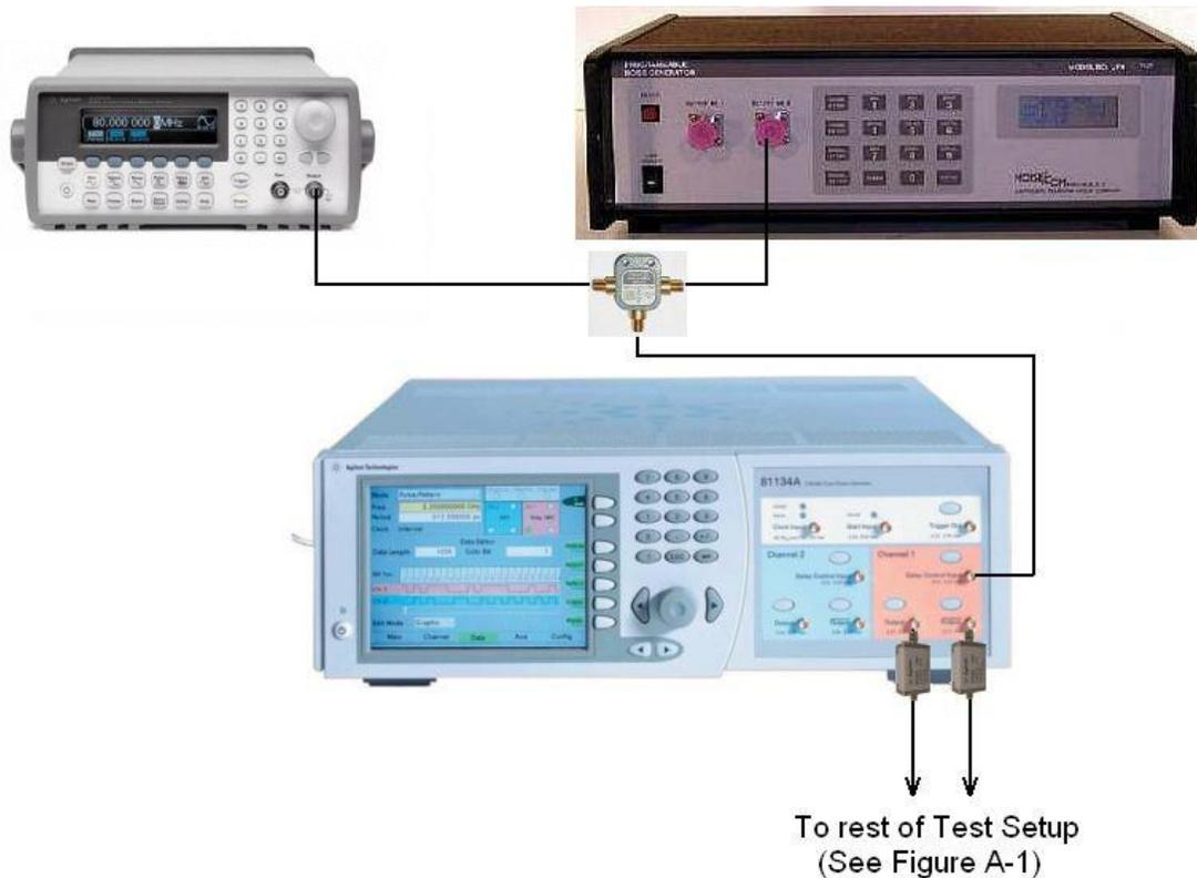
**Figure F-1: Agilent 81134A Pulse and Pattern Generator, Agilent 33250A Function/Arbitrary Waveform Generator, and Noisecom PNG-7110 Noise Generator**
