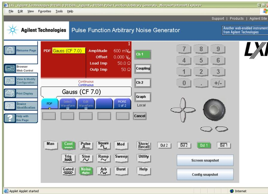
**Figure K-2: Agilent 81150A remote interface with noise settings for channel 1 shown. The LXI interface pictures the local user interface and all front panel controls.**
