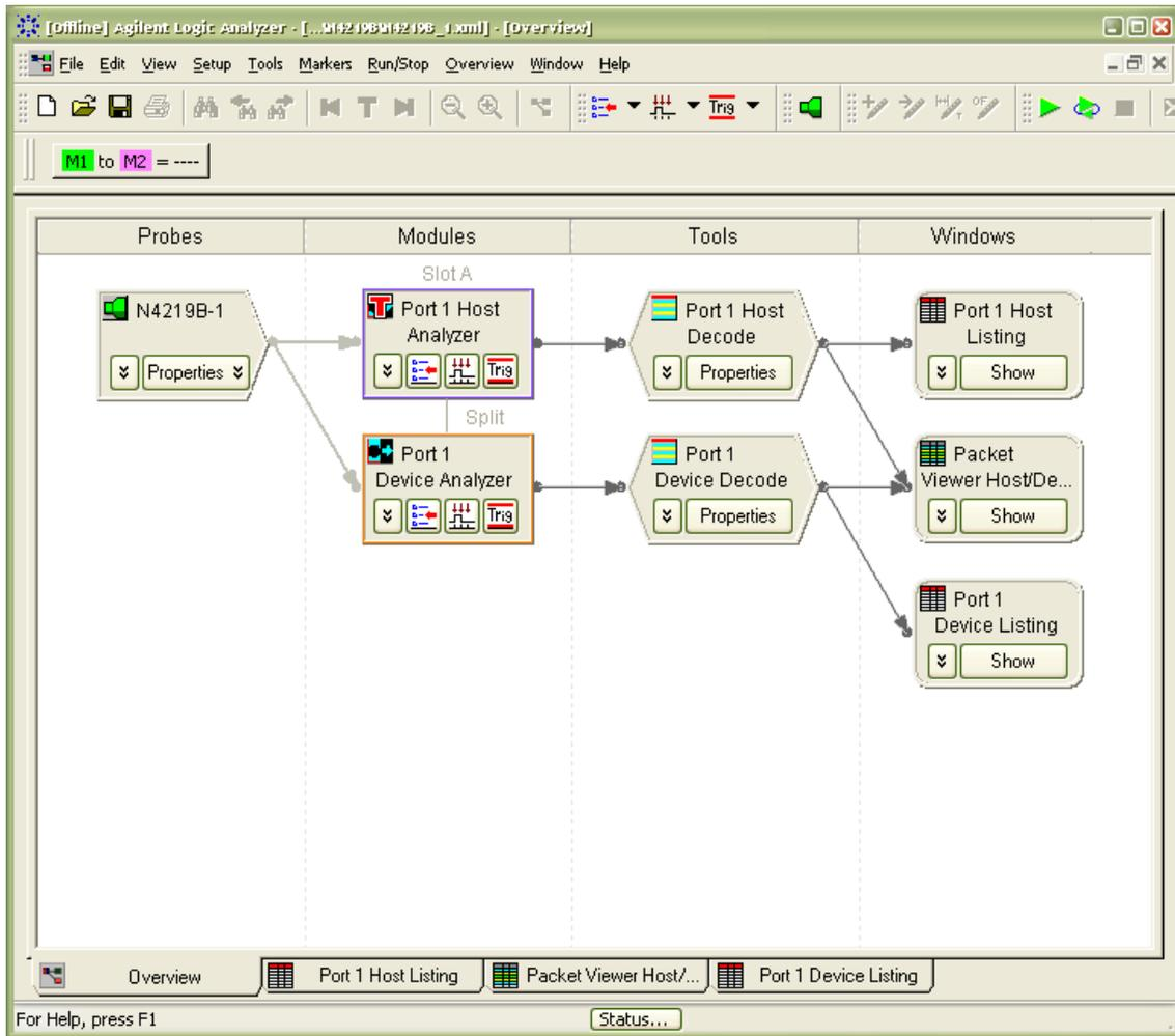
The Overview tab gives access to all required features for this test. For setup the N4219B Properties and the Port1 Device Analyzer Trigger will be configured later. When running the FER test the Status button at the bottom of this window will lead to the test results.
