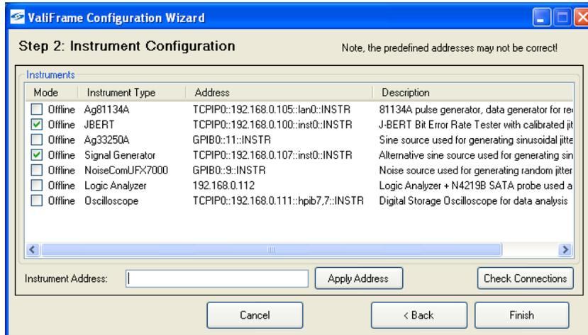
Offline Flags of J-BERT and Signal Generator should be checked. Offline flags for all other instruments should be unchecked. The addresses of the instruments must be changed. Press “Finish”.
