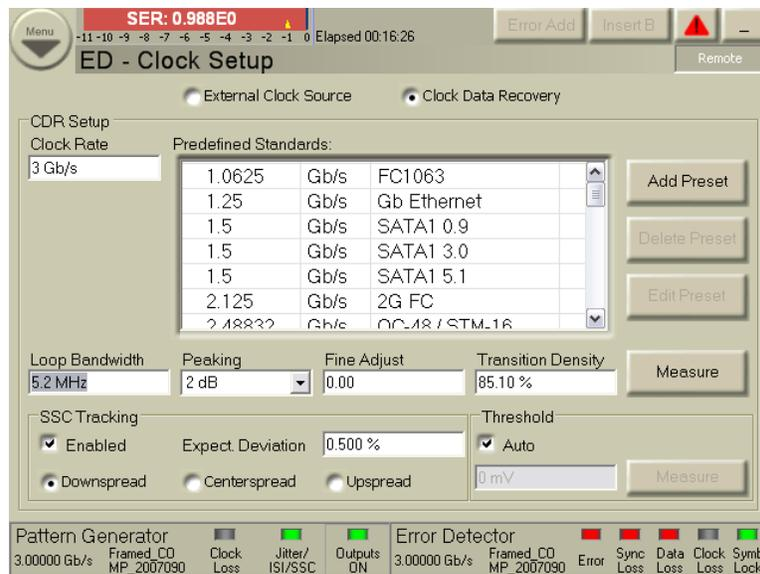
**Figure L-3: J-BERT Error Detector Clock Setup Menu**
