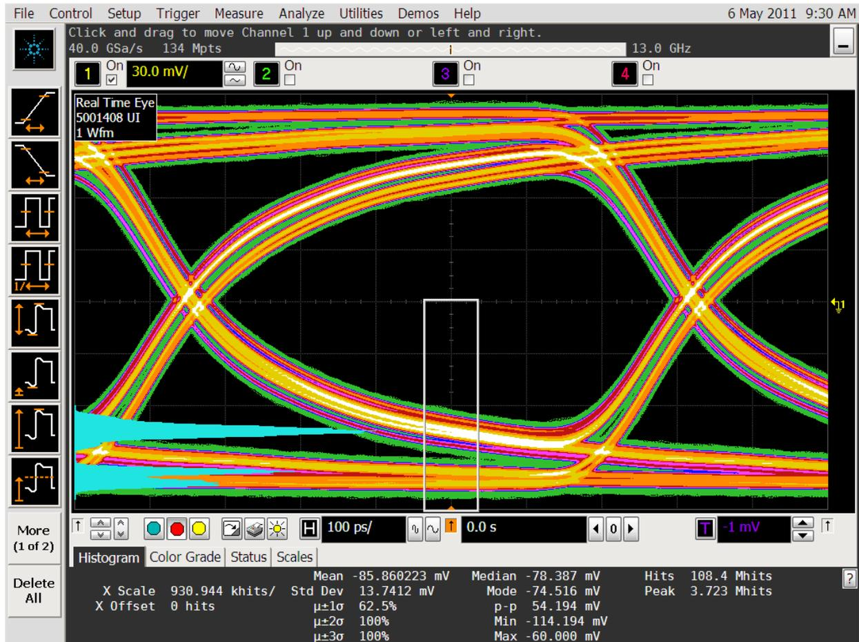
**Figure B-6: Gen1 Histogram Example for Lower Inner Eye (not calibrated)**
