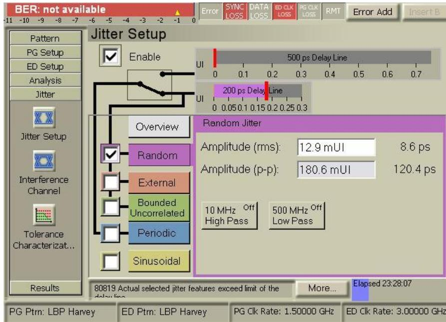
Figure E-3: J-BERTA Jitter Setup Screen (RJ)
