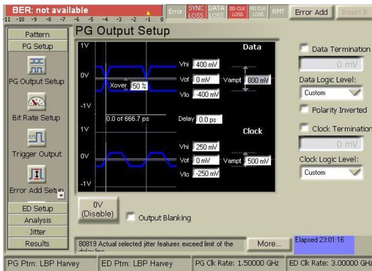
Figure E-2: J-BERTA Amplitude Setup Screen
