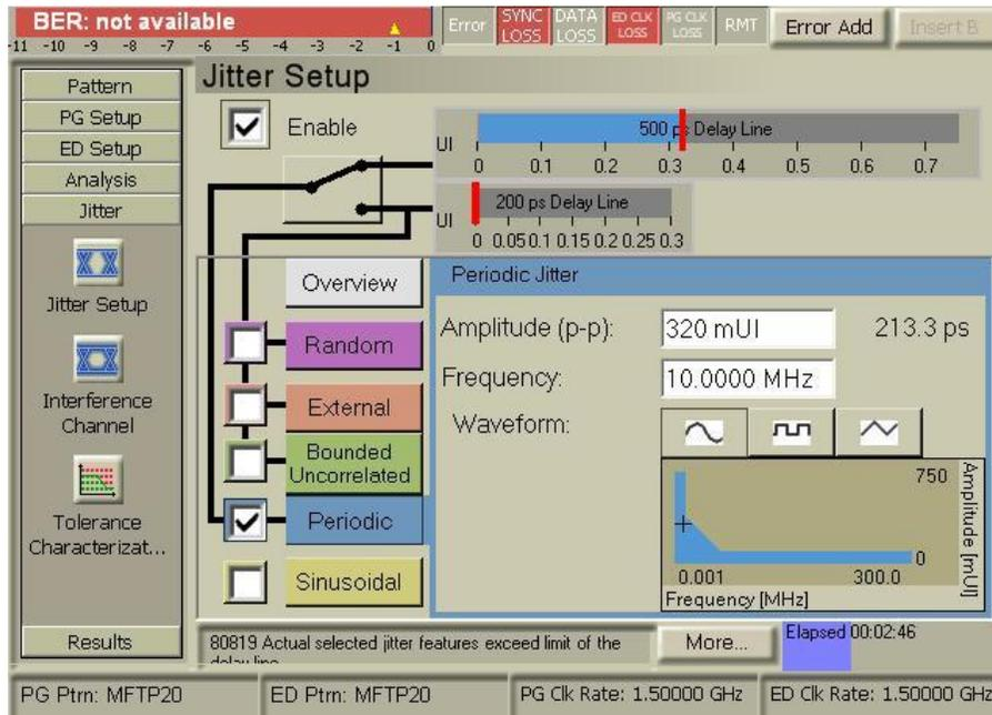
Figure E-4: J-BERTA Jitter Setup Screen (DJ)
