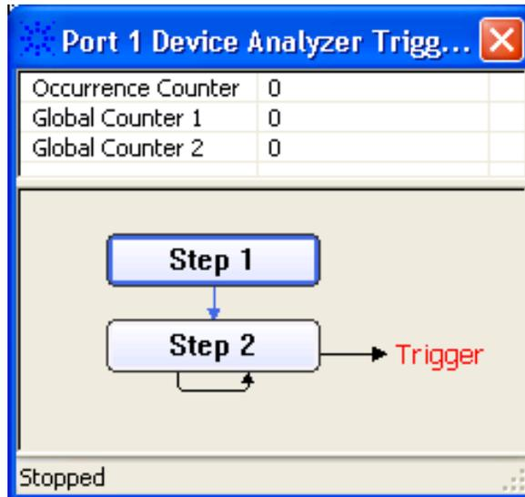
The Global Counter 1 values gives the actual number of FER errors in real-time while running the test. Based on the pass/fail criteria for RSG-01 and RSG-02 the test may be interrupted if the number of FERs reached its limit.
