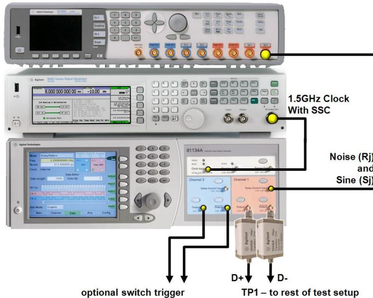
**Figure K-1: Agilent 81134A Pulse and Pattern Generator, Agilent 81150A Pulse Function Arbitrary Noise Generator, and Agilent N5182A MXG RF Vector Signal Generator**
