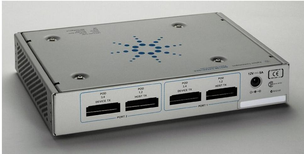
2. Make sure that POD 1, 2 and POD 3, 4 for Port 1 are connected to the logic analyzer. A connection for Port 2 is not required for this test.
