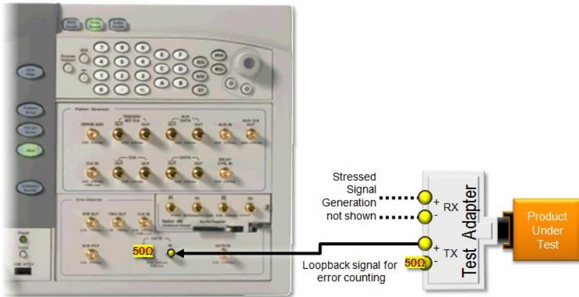
**Figure L-1: Connection Diagram Using J-BERT Error Detector as the Frame Error Detector**
