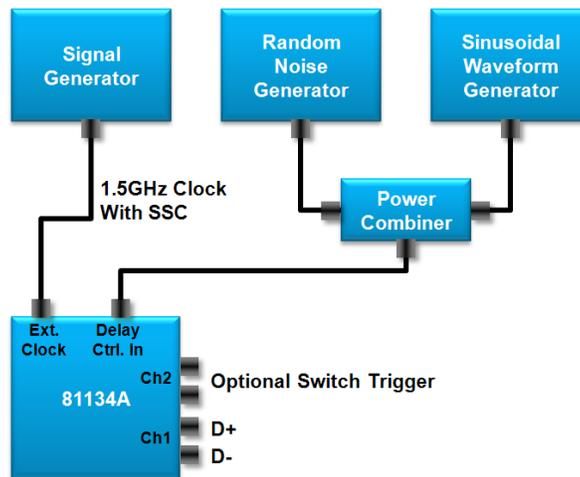
**Figure A-2: Use of Agilent 81133/4A as the SSG**
