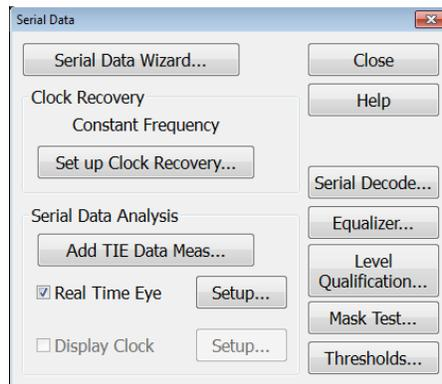
**Figure B-1: Enable Real Time Eye**
