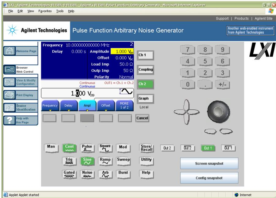
Figure K-4: Agilent 81150A remote interface with sinusoidal waveform configuration for channel 2 shown.
