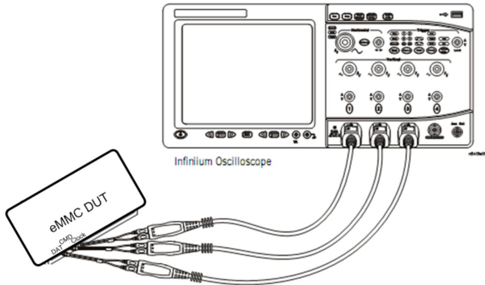
**Figure 10** Probing for HS200 Device Interface Timing Tests
