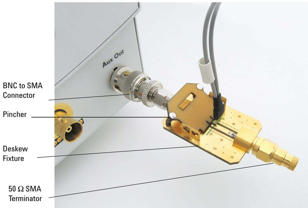
**Figure 17** Solder-in Probe Head Calibration Connection Example
