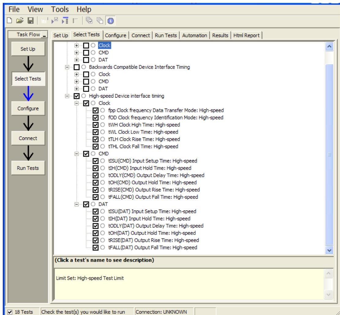
**Figure 7** Selecting High-Speed Device Interface Timing Tests
