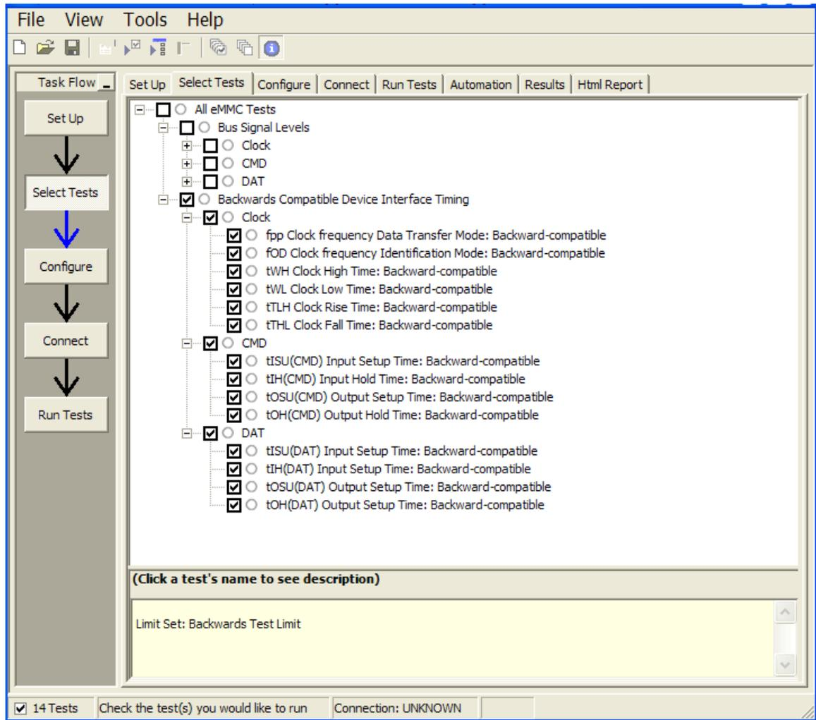
**Figure 5** Selecting Backwards Compatible Device Interface Timing Tests
