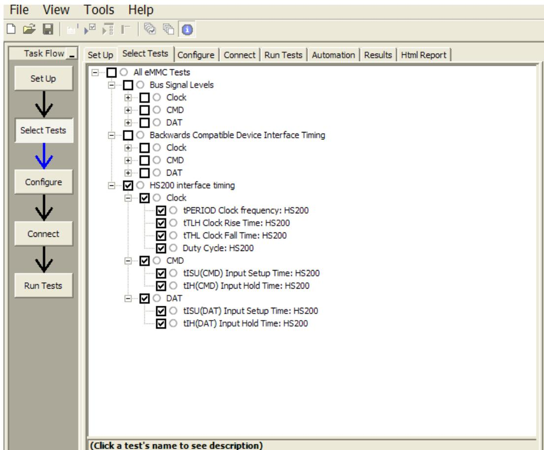
**Figure 11** Selecting HS200 Device Interface Timing Tests
