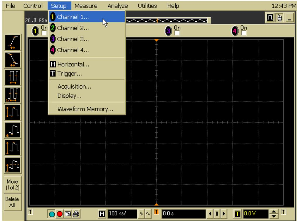
**Figure 20** Channel Setup Window
