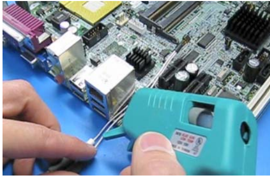
Figure 53 Probe Secured Using Low-Temperature Hot Glue
