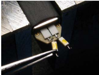
Figure 57 Soldering in a new axial resistor
