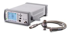
Keysight N432A, thermistor cable adaptor and thermistor sensors are all you need to perform accurate RF power measurements
