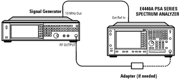
2. Verify that the spectrum analyzer is locked to the 10 MHz external reference frequency.
