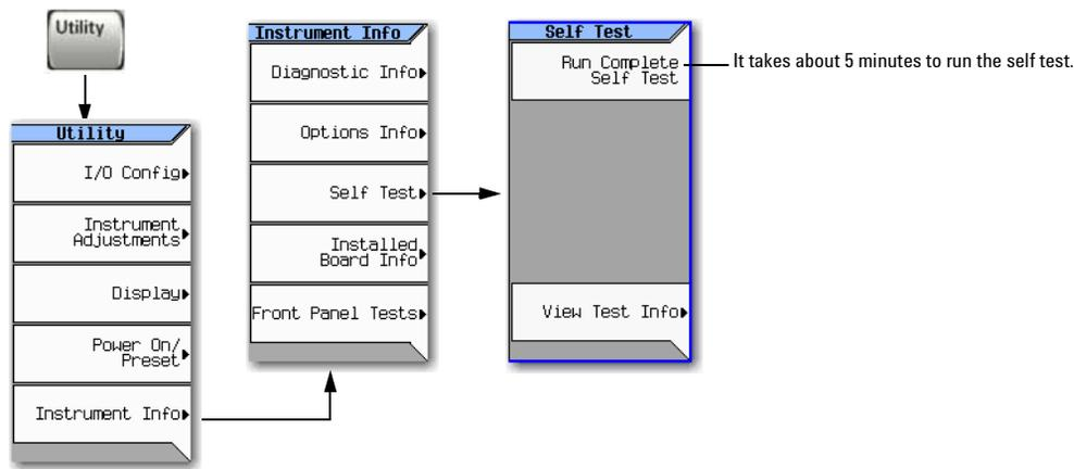
Use the following procedure to run self test:
