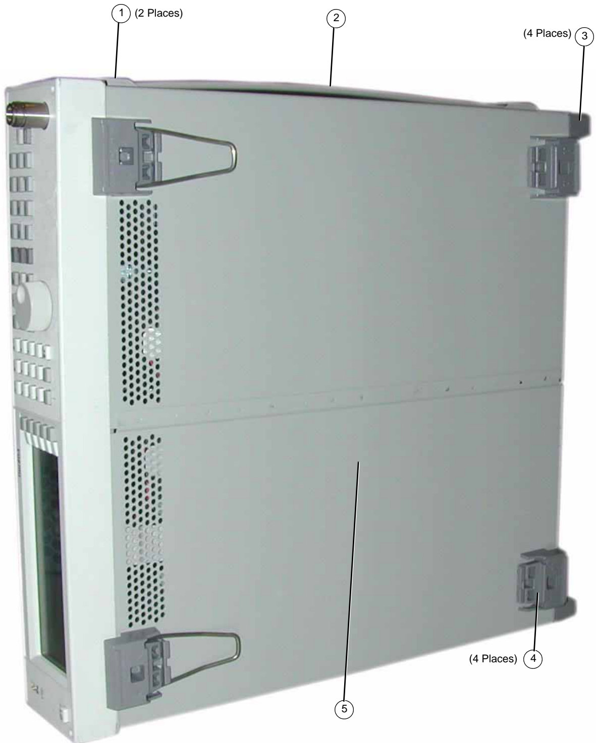
Figure 3-1 Outer Cover Removal
