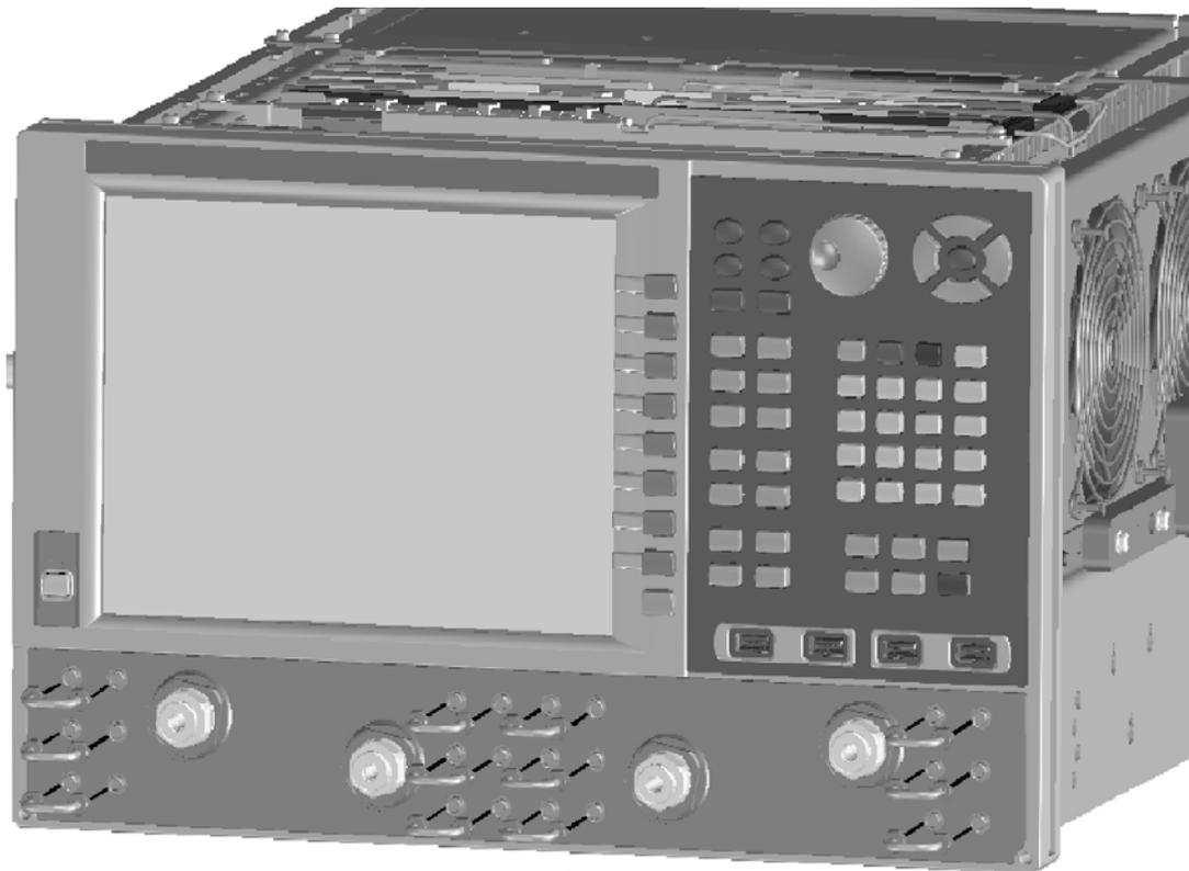
① Reinstall 12x jumper cables N5222-20091 and torque to 10 in-lbs.
